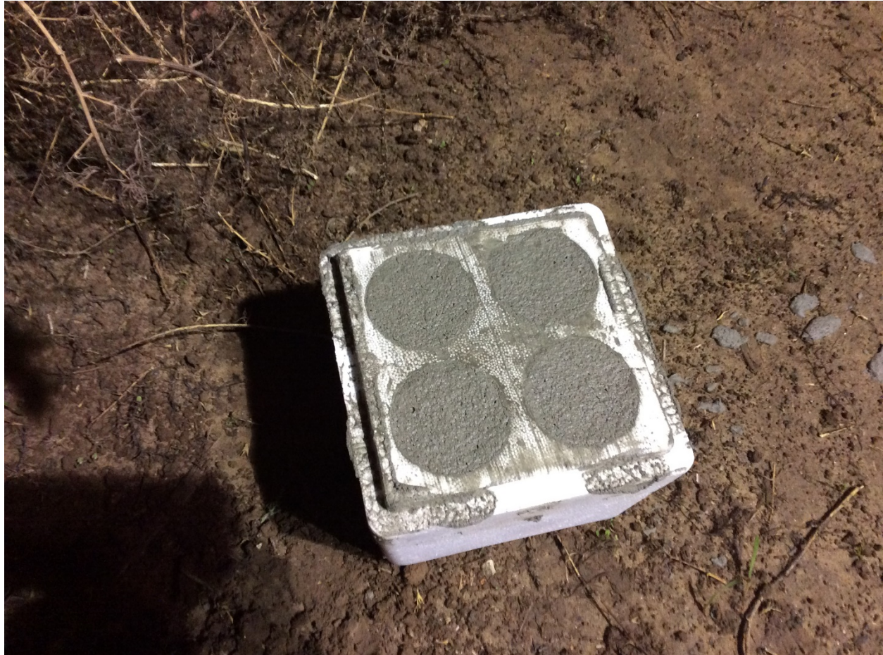
Figure 6: Grout Test Samples
