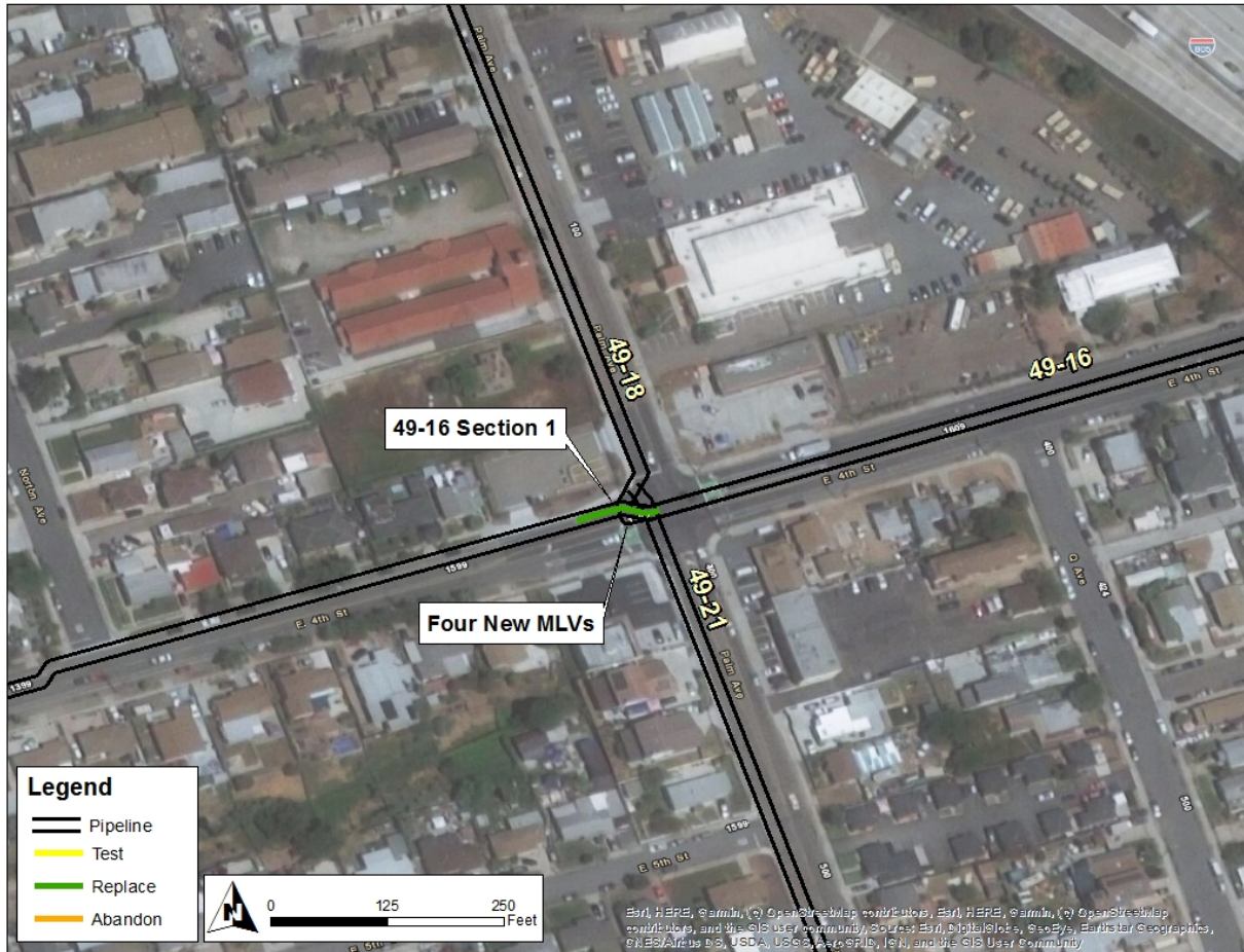
Figure 3: Satellite Image of Supply Line 49-16 Section 1 Replacement Project
