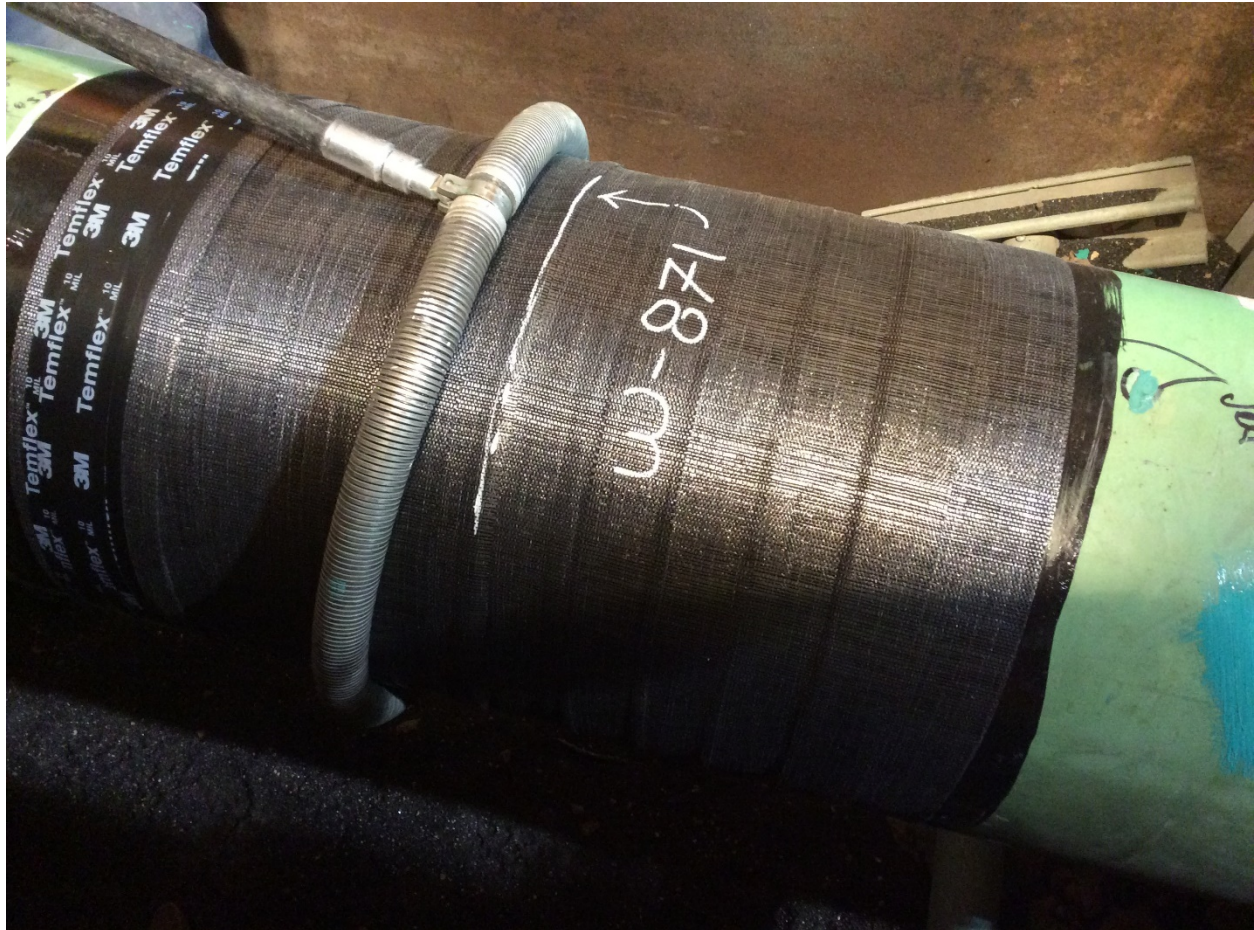
Figure 8: Holiday Testing of a Coated Weld
