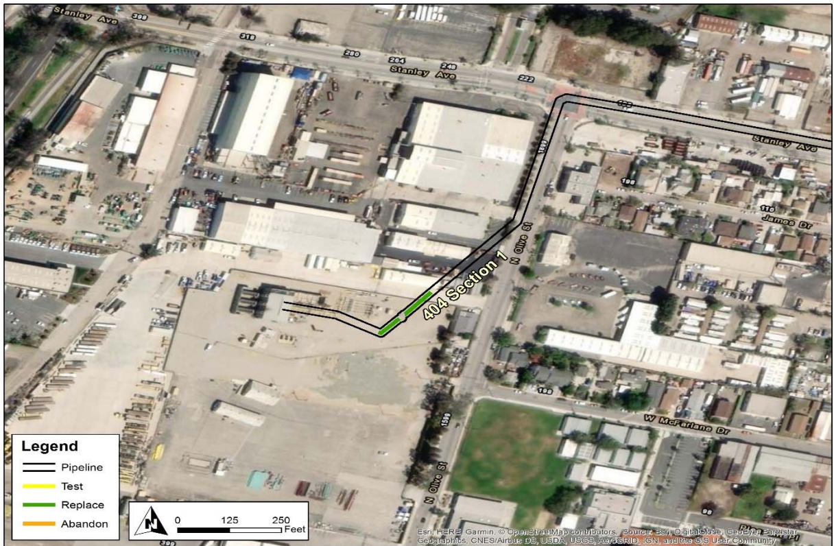
Figure 2: Satellite Image of Line 404 Section 1 Replacement Project
