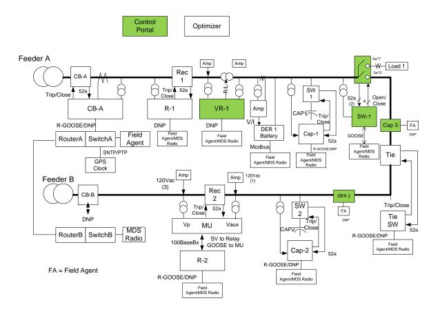
3.3 Test Case Diagram - UC 1a OpenFMB Connection to Relays & Virtual DER / Cap Bank
