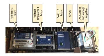
Figure 5 - Test System, Rack 2
