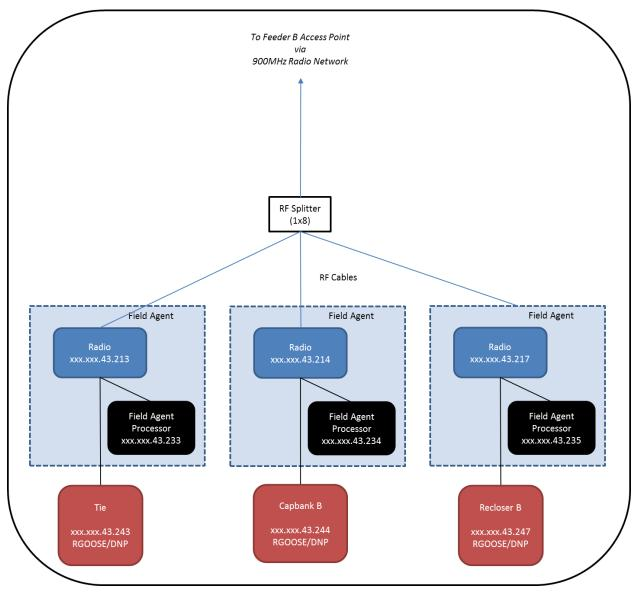
Figure 12 - Feeder B Remote Devices
