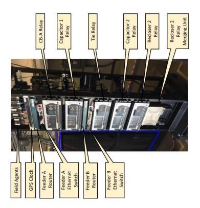
Figure 4 - Test System, Rack 1
