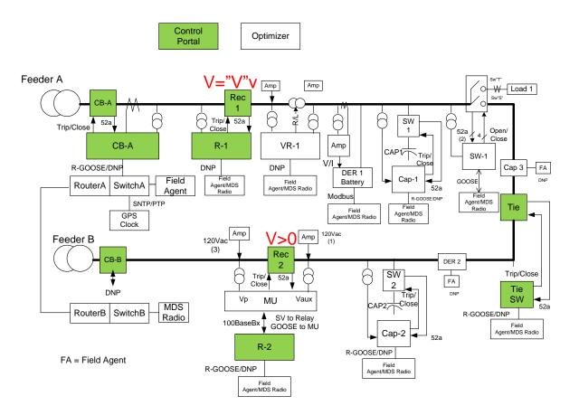
15.3 Use Case Diagram – UC 7a Automatic Feeder Re-Close (Use Case Diagram & Data Flow Summary redacted due to IP confidentiality concerns).
