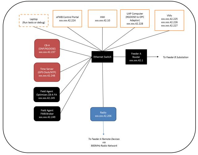
Figure 9 - Feeder A Substation Network
