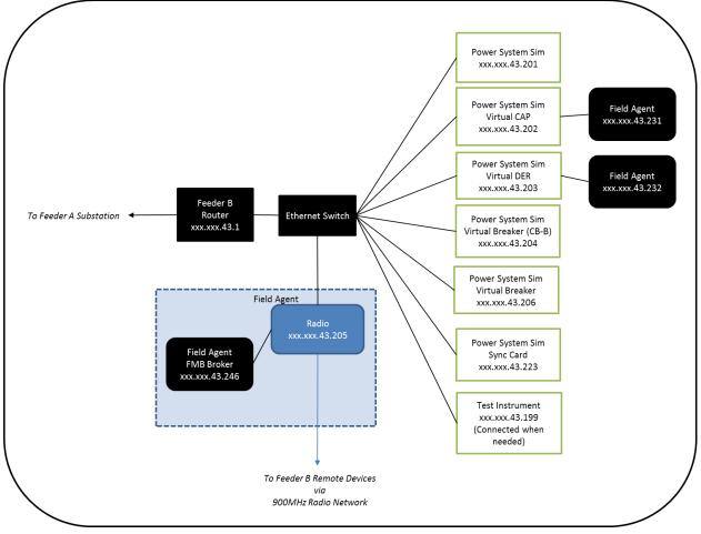
Figure 11 - Feeder B Substation Network
