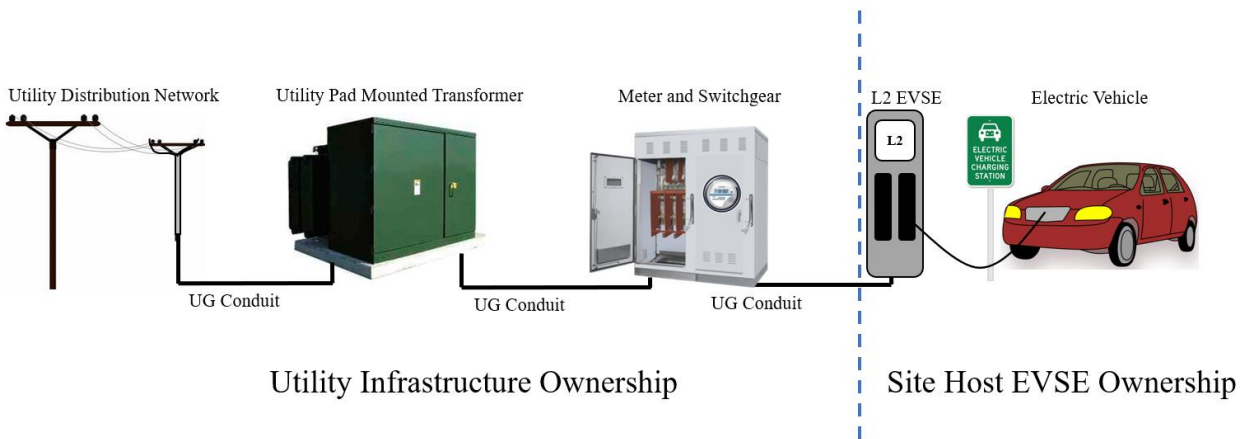
Figure 2-2: Power Your Drive Extension Program Architecture (Utility Owns Make-Ready Infrastructure and Workplace Site Host Owns EVSE)
