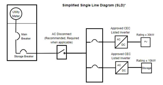
\*This Simplified SLD represents only equipment that is required by SDG&E for interconnection for this specific application. The AC output of an inverter could be connected directly to the service panel if an AC disconnect is not required.
