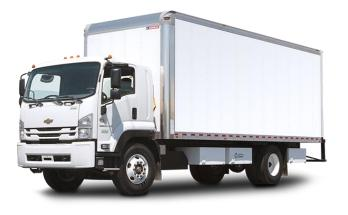
Sales Contact: Julie Johnson Enterprise Business Development julie.johnson@lightningsystems.com Weight Class (GVWR): Class 6 (19,501-26,000 lbs) Payload: 13,500 lbs Chassis/Body Type: Cab-over Energy Storage Capacity: 128-192 kWh Range: 88-130 miles Max Charge Rate: 80 kW Availability: In production
