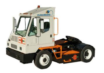
Weight Class (GVWR): Class 8 (33,001+ lbs) **Payload:** 81,000 lbs Chassis/Body Type: Yard Tractor Energy Storage Capacity: 80, 160 kWh **Range:** 50, 100 miles Max Charge Rate: 80 kW **Availability:** Production **Base Price:** \$200,000-\$280,000 Website: <u>https://orangeev.com/</u>
