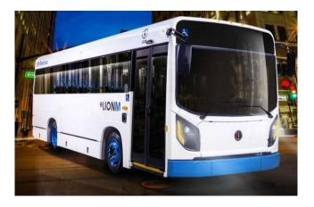
Sales Contact: Nate Baguio Vice President of Sales USA - Buses nate.baguio@thelionelectric.com Weight Class (GVWR): Class 6 (19,501-26,000) Passenger Capacity: 31 people Chassis/Body Type: Shuttle Bus Energy Storage Capacity: 160 kWh Range: 150 miles Max Charge Rate: 80 kW Availability: In production **Base Price:** \$290,000 Website: https://thelionelectric.com/en
