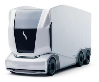
Weight Class (GVWR): Class 8 (33,001+ lbs) **Payload:** 35,000 lbs Chassis/Body Type: Tractor Energy Storage Capacity: 200-300 kWh Range: 80-186 miles Max Charge Rate: Not available **Availability:** In production **Base Price:** \$10,000 (monthly service fee up to \$22,500) Website: <u>https://www.einride.tech/</u>
