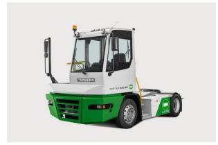
Sales Contact: Ron Van Arkel R.vanArkel@terbergamericas.com Weight Class (GVWR): Class 8 (33,001+ lbs) **Payload:** 130,000 Chassis/Body Type: Yard Tractor Energy Storage Capacity: 96, 148, 222 kW **Range:** 5.5, 8, 12 hours Max Charge Rate: 96 kW Availability: In production Base Price: \$270,000-\$355,000 Website: https://www.terbergtractorsamericas.com/en/
