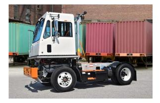
Weight Class (GVWR): Class 8 (33,001+ lbs) **Payload:** 42,000 Chassis/Body Type: Yard Tractor Energy Storage Capacity: 132, 172, 196 kW Range: Not available Max Charge Rate: Not available Availability: Pre-production **Base Price:** \$275,000–\$310,000 Website: http://ticotractors.com/pro-spotter/
