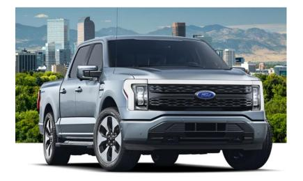
Weight Class (GVWR): Class 2 (6,001-10,000 lbs) **Payload:** 2,000 lbs Chassis/Body Type: Pickup **Energy Storage Capacity:** Not available **Range:** 230-300 miles Max Charge Rate: 19.2 kW Availability: In production **Base Price:** \$39,974 Website: https://www.ford.com/...
