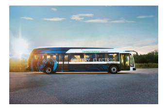
Sales Contact: Bill Williams Director, Commercial Sales bwilliams@proterra.com Weight Class (GVWR): Class 8 (33,001+ lbs) Passenger Capacity: 40 people **Chassis/Body Type:** Transit Bus Energy Storage Capacity: 675 kWh **Range:** 205-329 miles Max Charge Rate: 135 kW (plug in); 407 kW (overhead) Availability: In production **Base Price:** Not available Website: <u>https://www.proterra.com/</u>
