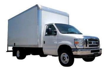
Weight Class (GVWR): Class 4 (14,001-16,000 lb) Payload: 5,088 lbs Chassis/Body Type: Cutaway Energy Storage Capacity: 108, 144 kWh Range: 100-125 miles Max Charge Rate: Not available **Availability:** Pre-production **Base Price:** \$211,000 Website: <u>https://www.alphamobility.co/</u>
