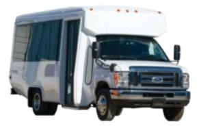
Weight Class (GVWR): Class 4 (14,001-16,000 lbs) Passenger Capacity: 25 people Chassis/Body Type: Shuttle Bus Energy Storage Capacity: 108 kWh, 144 kWh Range: 100-125 miles Max Charge Rate: Not available **Availability:** Pre-production **Base Price:** \$222,000
