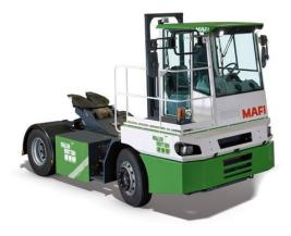
Weight Class (GVWR): Class 8 (33,001+ lbs) **Payload:** 198,000 lbs (GCW) Chassis/Body Type: Yard Tractor Energy Storage Capacity: 177 kW **Range:** Not available Max Charge Rate: Not available Availability: In production **Base Price:** Not available Website: https://www.mafi.de/en/products/tractors/electric-
