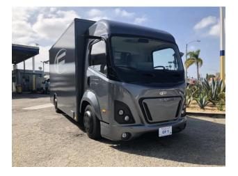
Weight Class (GVWR): Class 3 (10,001-14,000 lb) **Payload:** 4,800 lbs **Chassis/Body Type:** Straight/Box Truck Energy Storage Capacity: Not available Range: 100 miles Max Charge Rate: Not available **Availability:** Pre-production **Base Price:** Not available Website: <u>https://www.cityfreighter.com/</u>
