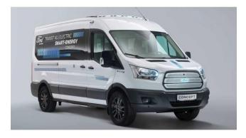
Weight Class (GVWR): Class 2 (6,001-10,000 lbs) Payload: 4,290-3,800 lbs Chassis/Body Type: Cutaway, Cab Chassis, Van Energy Storage Capacity: 67 kWh Range: 126 miles Max Charge Rate: 115 kW **Availability:** Production **Base Price:** \$45,000
