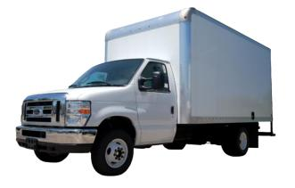
Weight Class (GVWR): Class 4 (14,001-16,000 lb) Payload: 6,900-6,100 lbs **Chassis/Body Type:** Straight/Box Truck Energy Storage Capacity: 151 kWh Range: 135 miles Max Charge Rate: 180 kW Availability: In production **Base Price:** \$173,598
