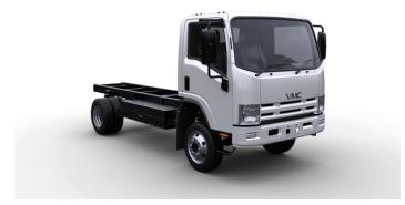
Weight Class (GVWR): Class 3 (10,001-14,000 lbs) **Payload:** 6,000 lbs **Chassis/Body Type:** Straight/Box Truck Energy Storage Capacity: 150 kWh Range: 180 miles Max Charge Rate: 50 kW Availability: In production **Base Price:** Not available Website: https://vmctrucks.com/
