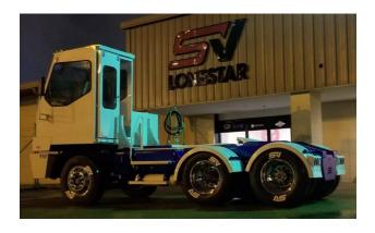
Weight Class (GVWR): Class 8 (33,001+ lbs) Payload: Not available Chassis/Body Type: Yard Tractor Energy Storage Capacity: 112 kWh, 220 kWh Range: 12-22 hours Max Charge Rate: 163 kW Availability: In production **Base Price:** \$215,000-\$265,000 Website: https://www.lonestarsv.com/4x2models
