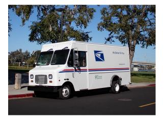
Sales Contact: John Felts Sales Representative NorCal & NW USA john.felts@motivps.com Weight Class (GVWR): Class 4 (14,000-16,000 lbs) Payload: 5,000-6,000 lbs Chassis/Body Type: Cutaway, Stripped Chassis Energy Storage Capacity: 127 kWh Range: 105 miles
