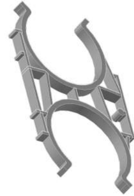
FIGURE 3 5-INCH VERTICAL SPACER FOR 9-INCH WIDTH TRENCH
