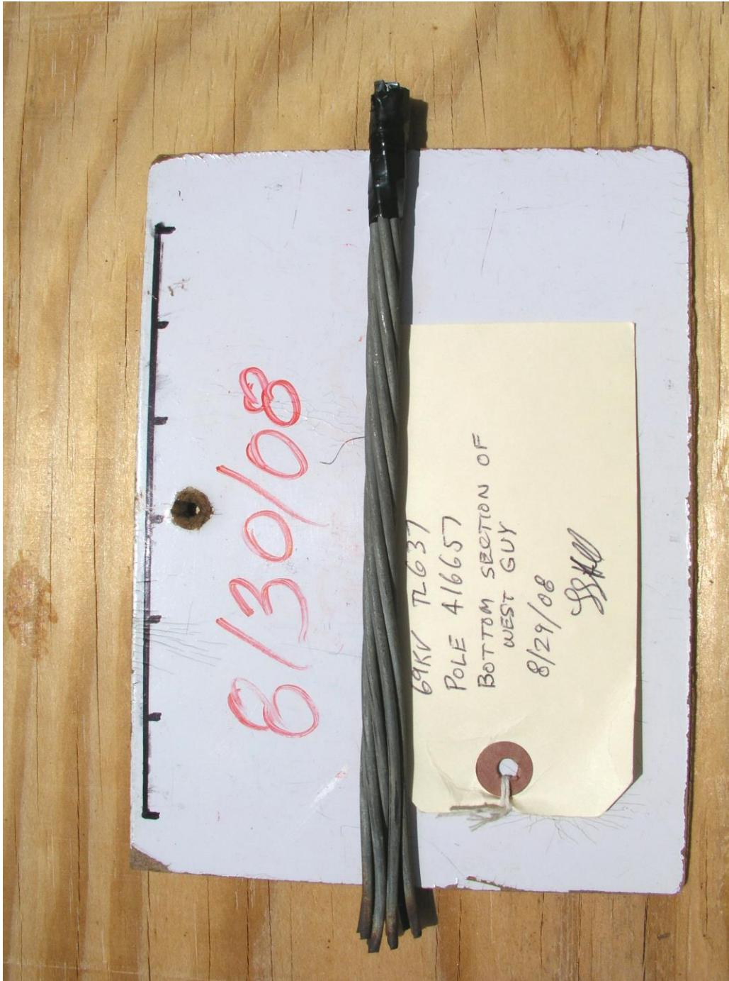
Figure 1. Guy wire sample removed from West guy
