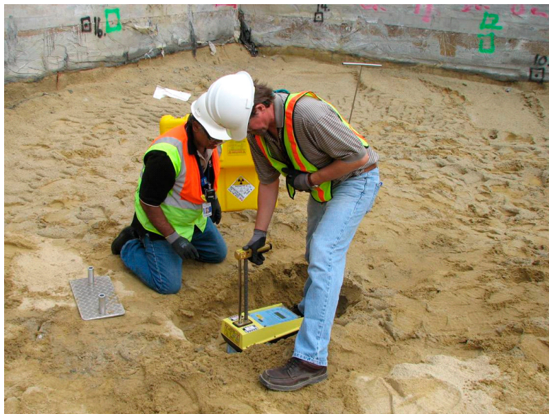
Figure III-35 Performing Soil Compaction Testing in SONGS 1 Yard Area
