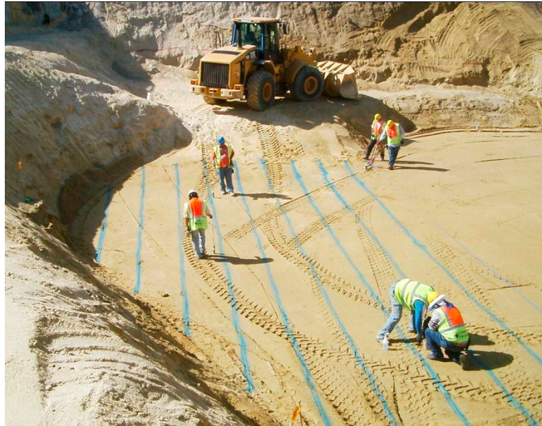
Figure III-35 Performing Soil Compaction Testing in SONGS 1 Yard Area
