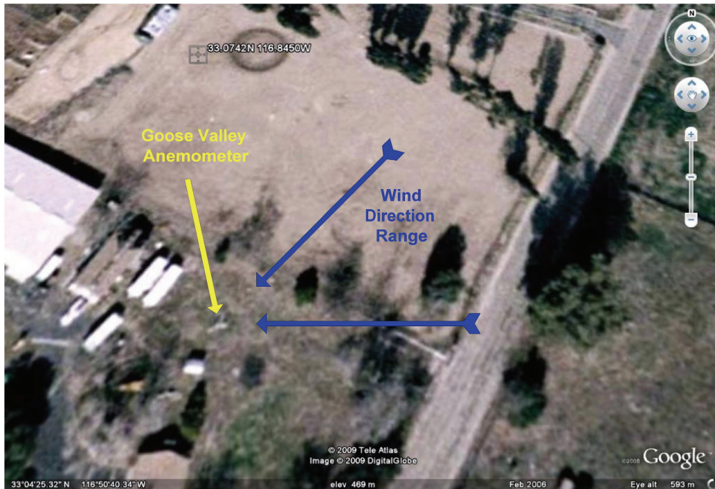
Exhibit 15b. Goose Valley anemometer location with wind direction range during the Santa Ana event; note sheltering trees upwind of anemometer.
