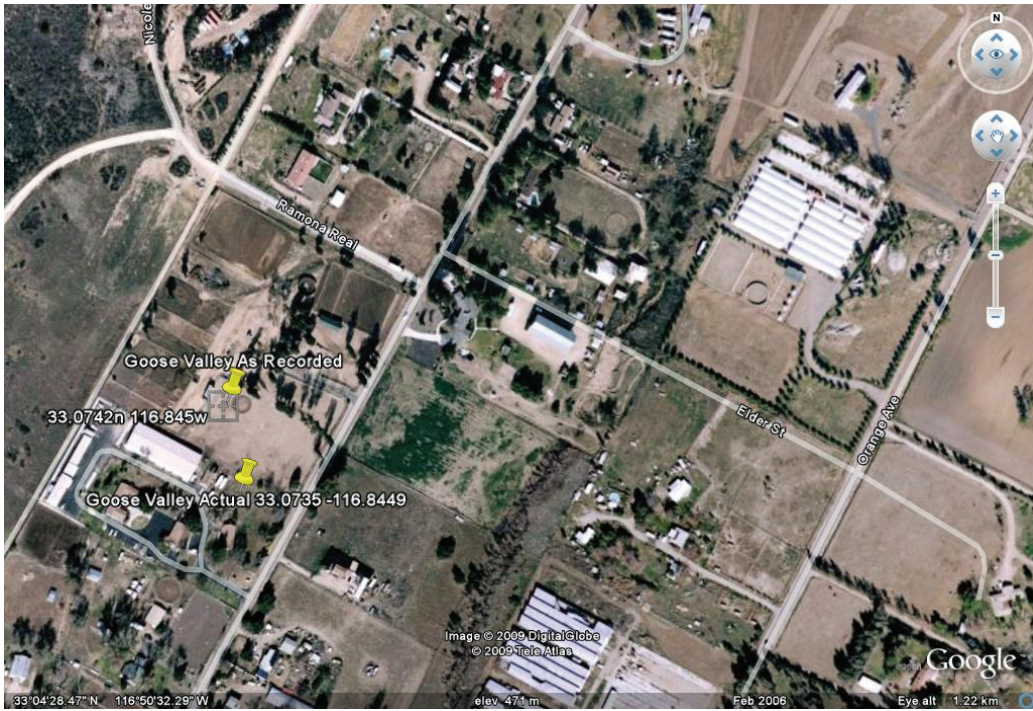
Exhibit 15a. Goose Valley anemometer location as recorded and the actual location; note sheltering buildings and trees to the east-northeast.
