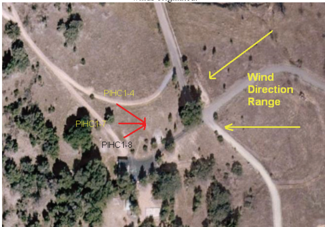
Exhibit 13b. Pine Hills anemometer location and location of photographs PIHC1-4, PIHC1-7, and PIHC1-8 with wind direction range during the Santa Ana event; note the large tree directly upwind of the anemometer.
