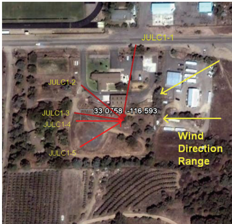
Exhibit 10b. Julian anemometer location and location of photographs JULC1-1, JULC1-2, JULC1-3, JULC1-4, and JULC1-5 with wind direction range during the Santa Ana event; note sheltering trees and structures upwind of anemometer.
