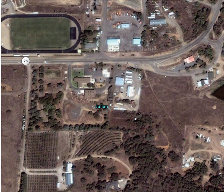
Exhibit 10a. Julian anemometer location; note sheltering trees and structures surrounding site on all sides.
