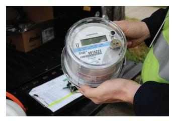
Smart meters will be installed towards the front of the home to provide quick and safe access to SDG&E crew, emergency crew and first responders.
