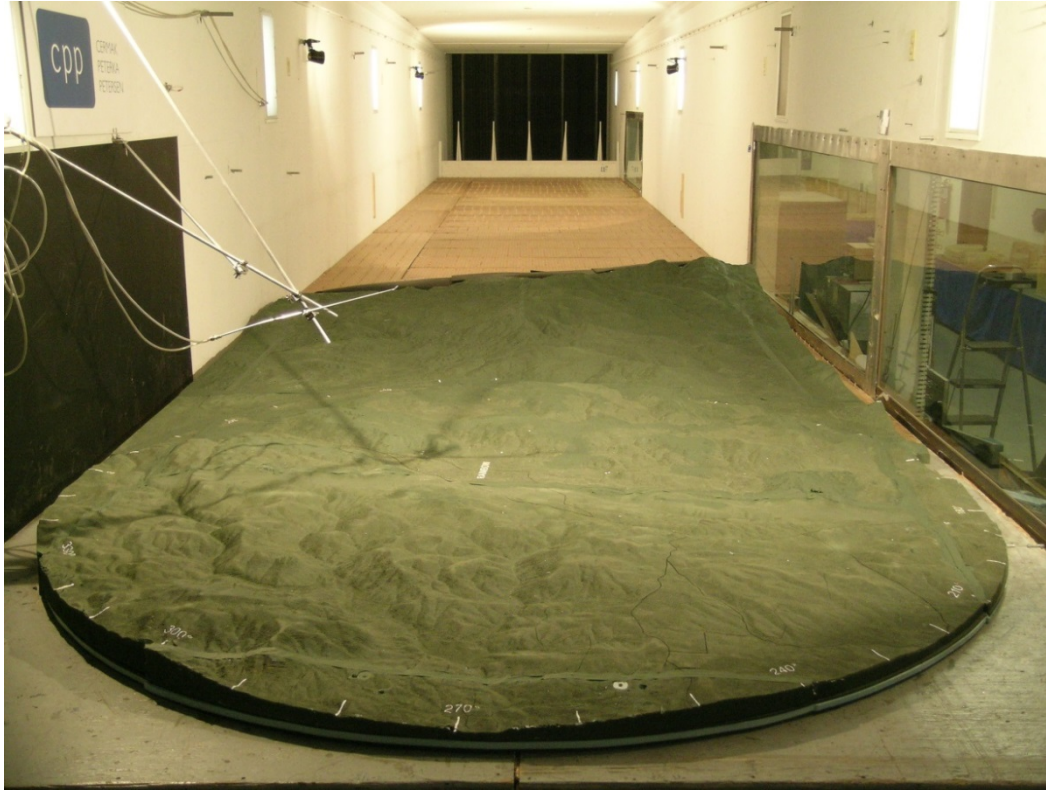
Appendix 3e. Rice Canyon wind tunnel model test turntable with upwind terrain.
