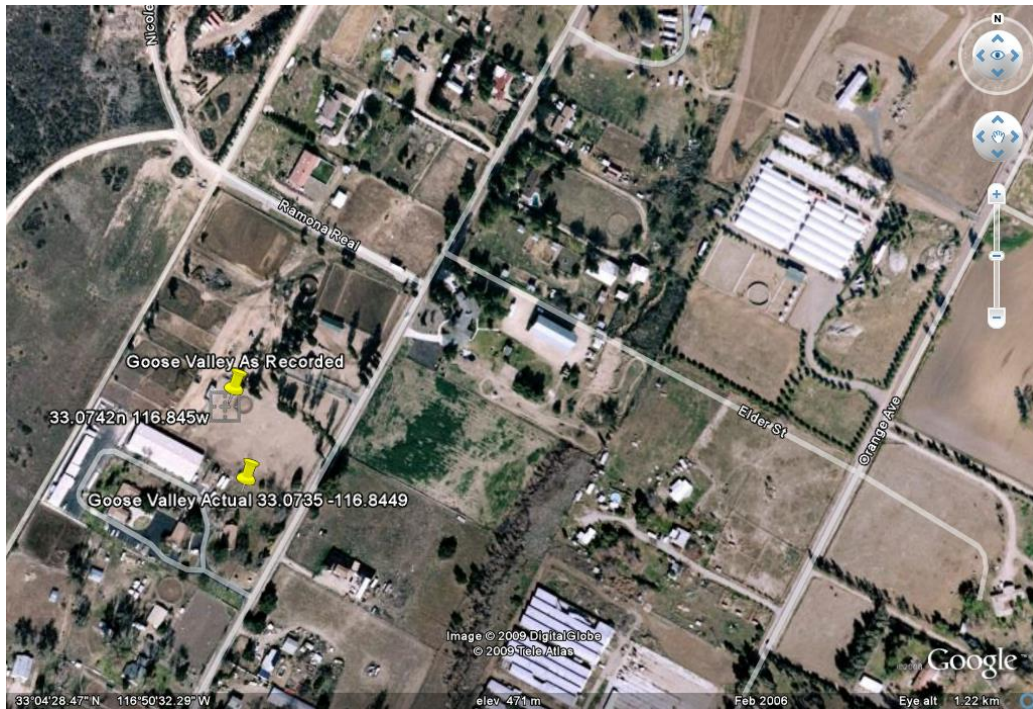
Appendix 15a. Goose Valley anemometer location as recorded and the actual location; note sheltering buildings and trees to the east-northeast.
