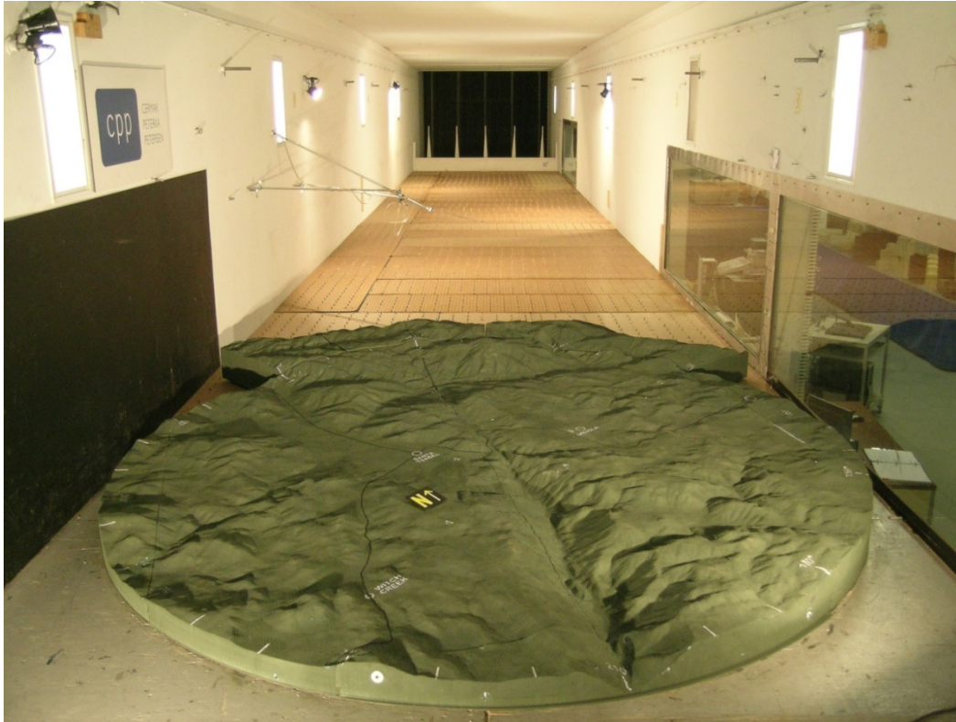
Appendix 3a. Witch Creek wind tunnel model test turntable with upwind terrain.
