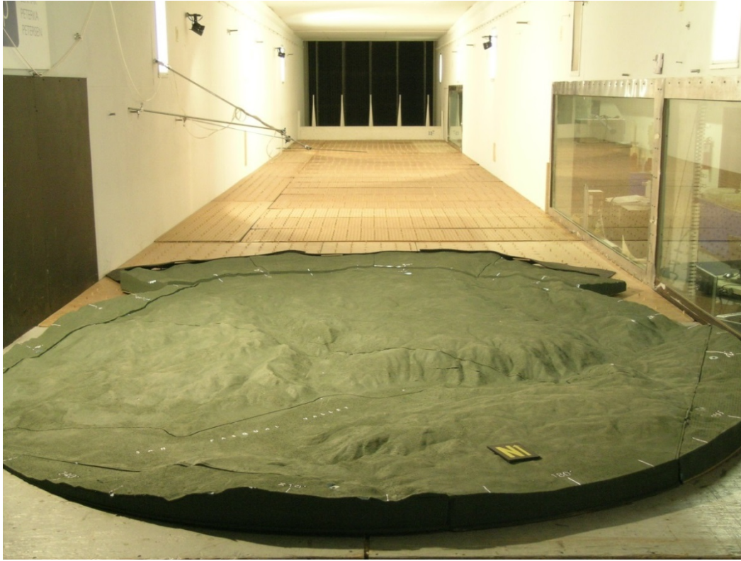
Appendix 3c. Guejito wind tunnel model test turntable with upwind terrain.
