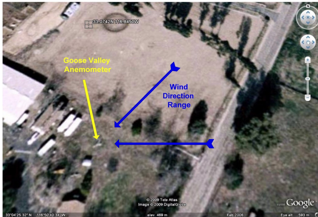
Appendix 15b. Goose Valley anemometer location with wind direction range during the Santa Ana event; note sheltering trees upwind of anemometer.
