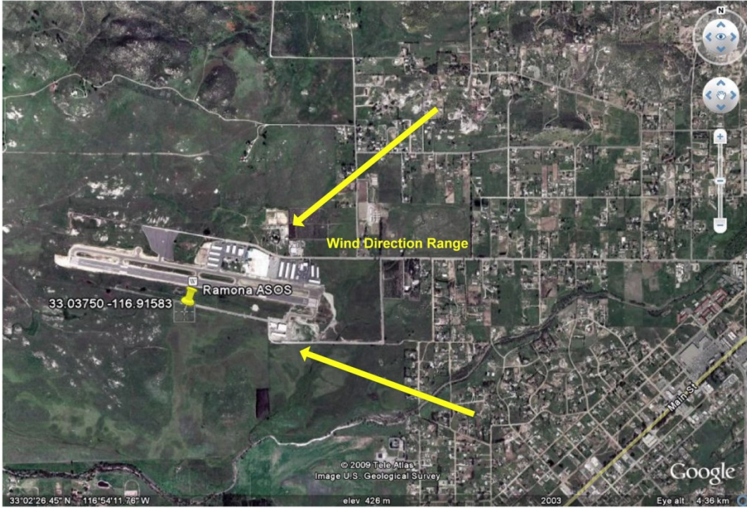
Appendix 17a. Ramona Airport ASOS station location. Note suburban development upwind for the storm event and airport hangar buildings upwind causing some shielding. Refer to Appendix 12 for another view and refer to discussion of Appendix 12.
