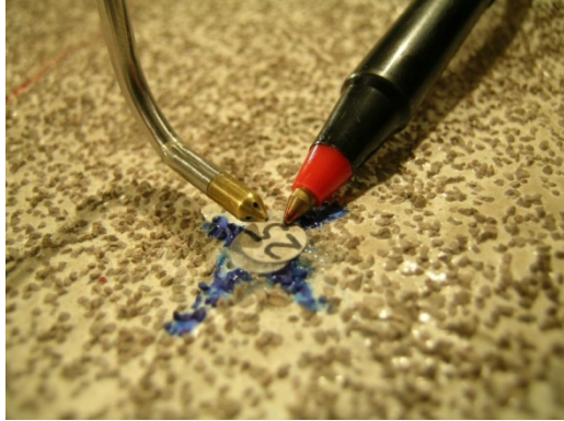
Appendix 3g. Measurement probe to sample 3 components of velocity on all three models.
