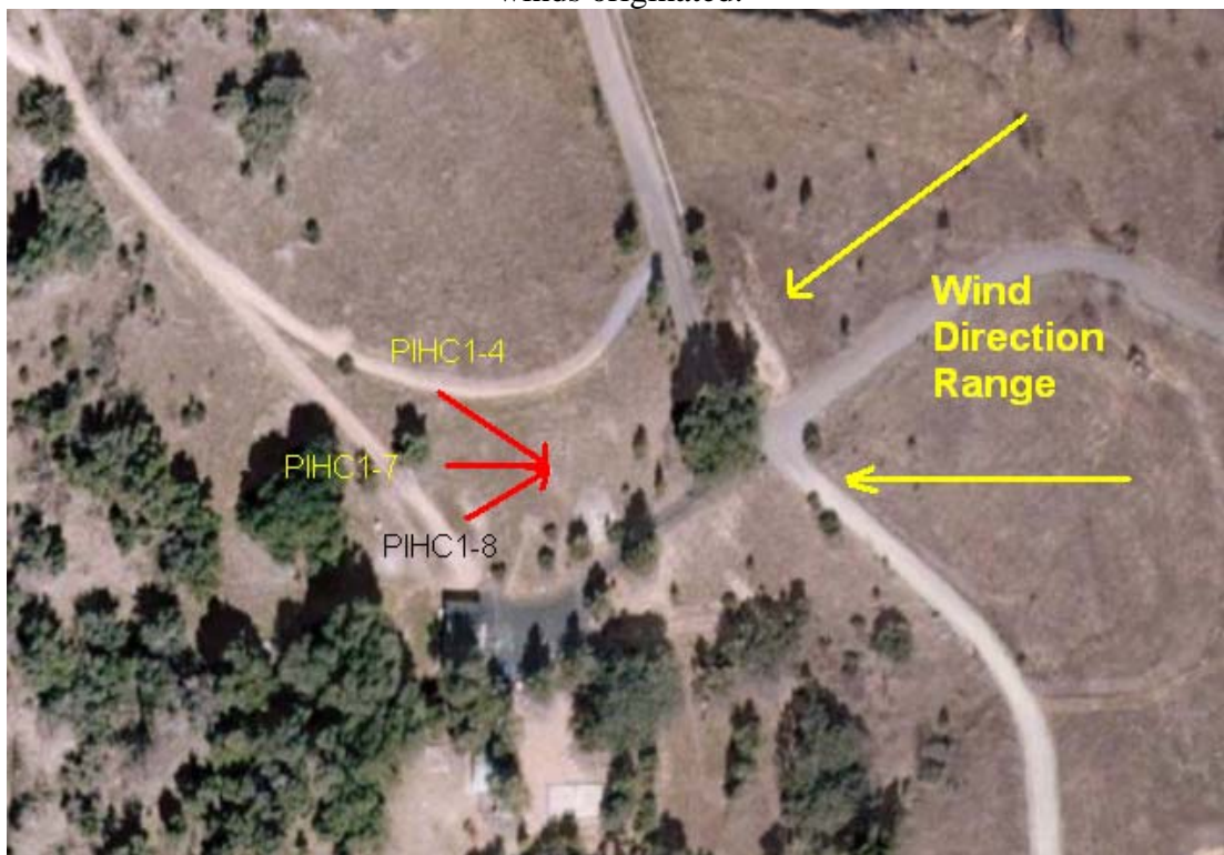
Appendix 14b. Pine Hills anemometer location and location of photographs PIHC1-4, PIHC1-7, and PIHC1-8 with wind direction range during the Santa Ana event; note the large tree directly upwind of the anemometer.
