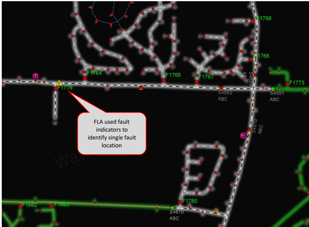
Fig. 10. FLA graphical results with WFI analysis
