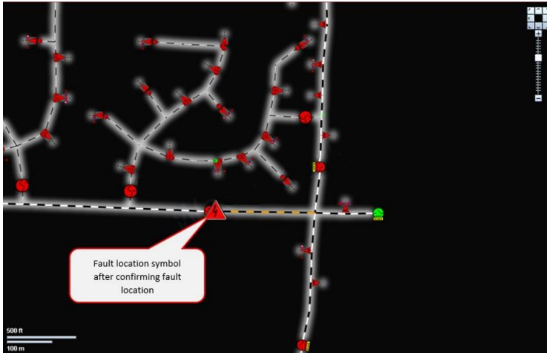
Fig. 7. FLA Results After Confirming Actual Fault Location
