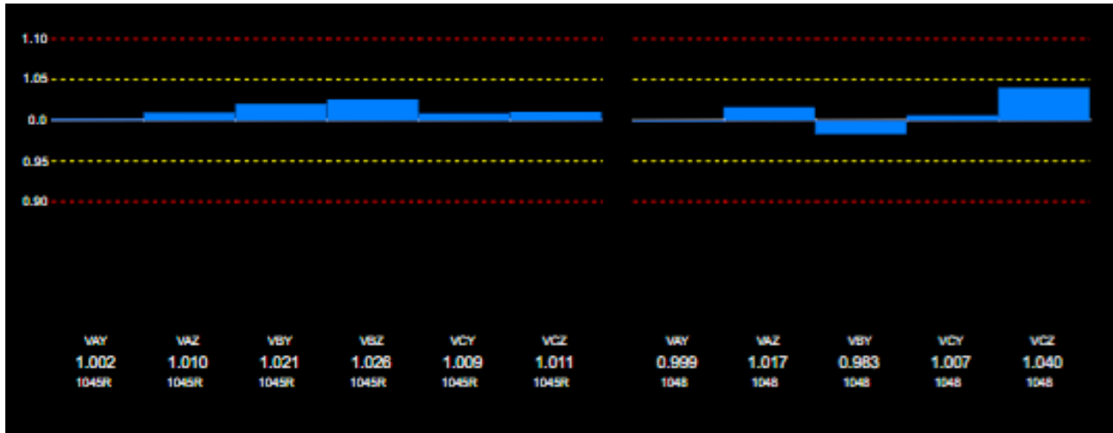
Figure 3-12. Voltage deviations (from base voltage) in percentage along the selected circuit length (circuit 1)
