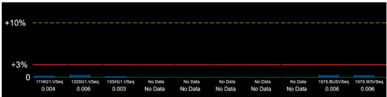
Figure 3-2. Monitoring of voltage unbalance factor
