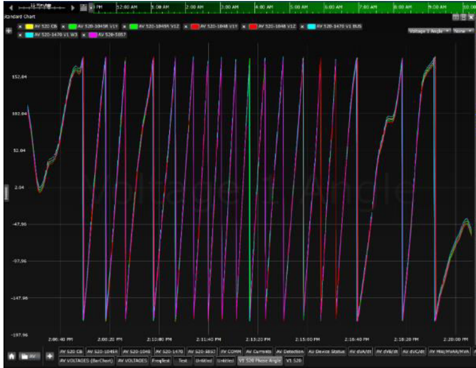
Figure 3-13. Voltage phase angle in phasor time domain
