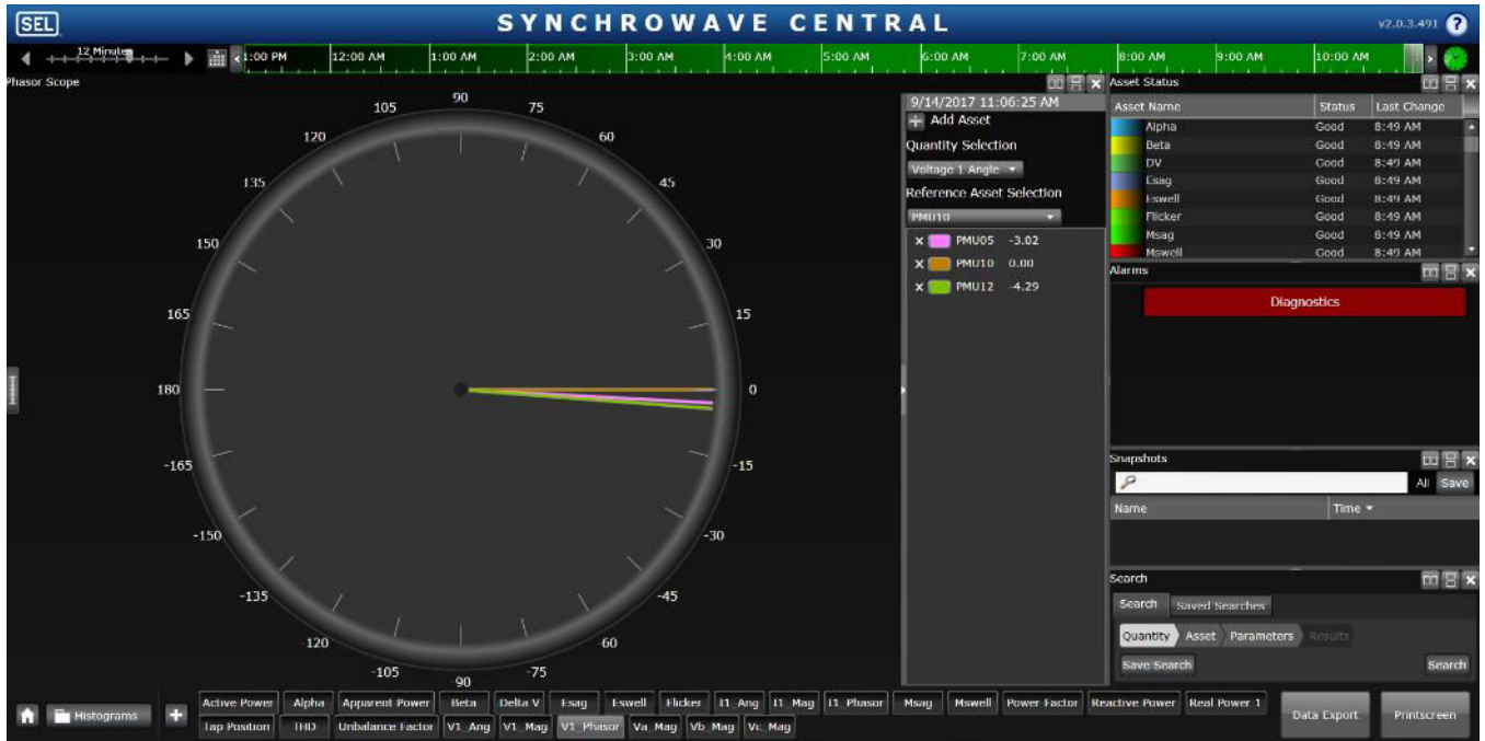
Figure 4-12. Phase Angles of the Two Sides of the 520-1048 during Low Loading without PV.
