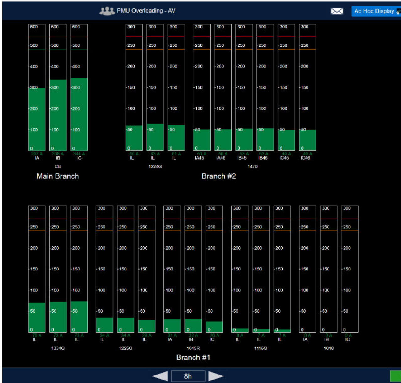
Figure 3-7. Thermal loading asset monitoring on Main branch, Branch #1 and Branch #2 of the Circuit 1
