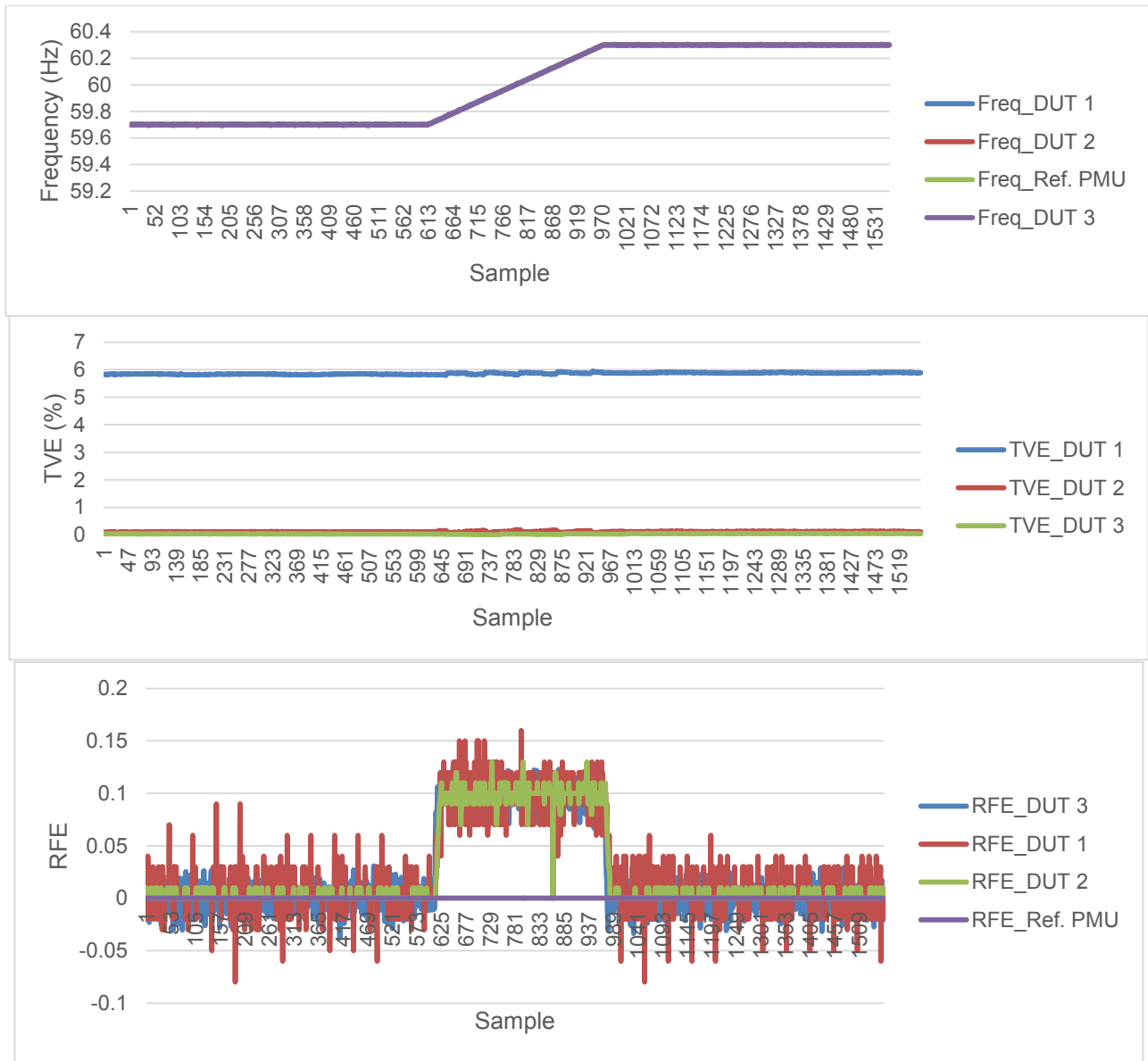
Figure 2-27. Frequency, TVE, and RFE Subsequent to Frequency Ramp (Case 2-2-1)
