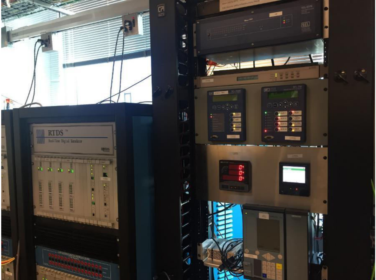
Figure 2-6. PMU Test Setup at the ITF lab
