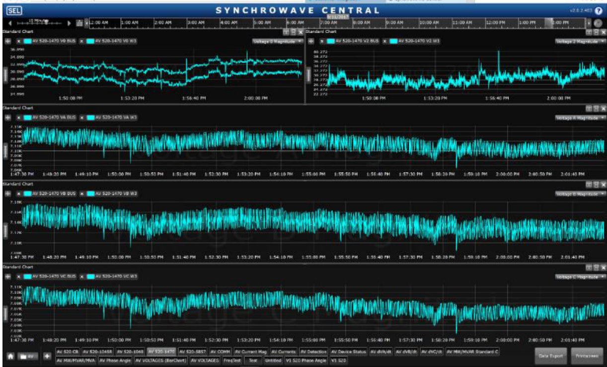
Figure 3-15. Voltage magnitude of the Circuit 1 PMUs (standard view)
