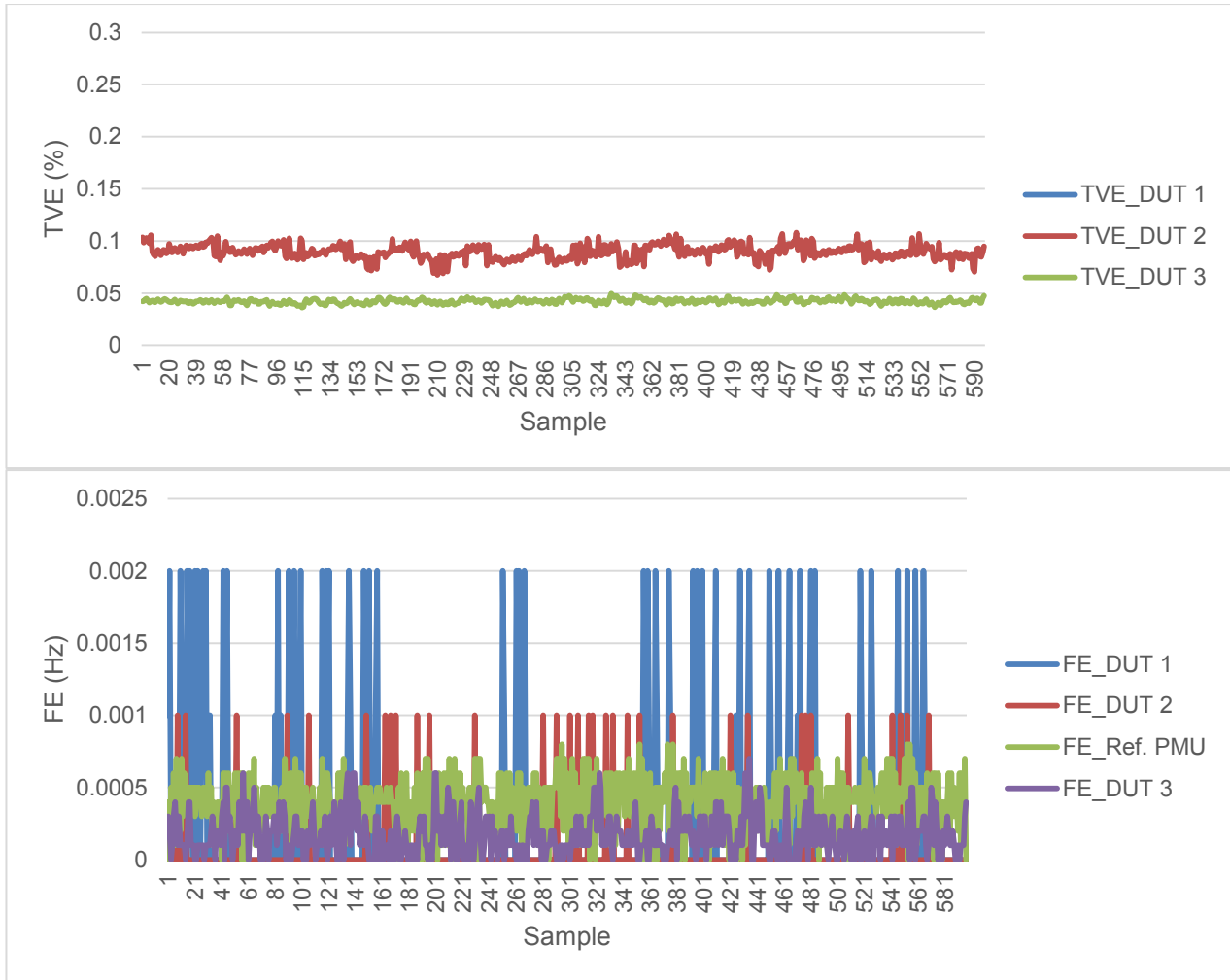
Figure 2-18. TVE and FE during the Injection of 3% Magnitude of 5th Harmonic (Case 1-3-1)
