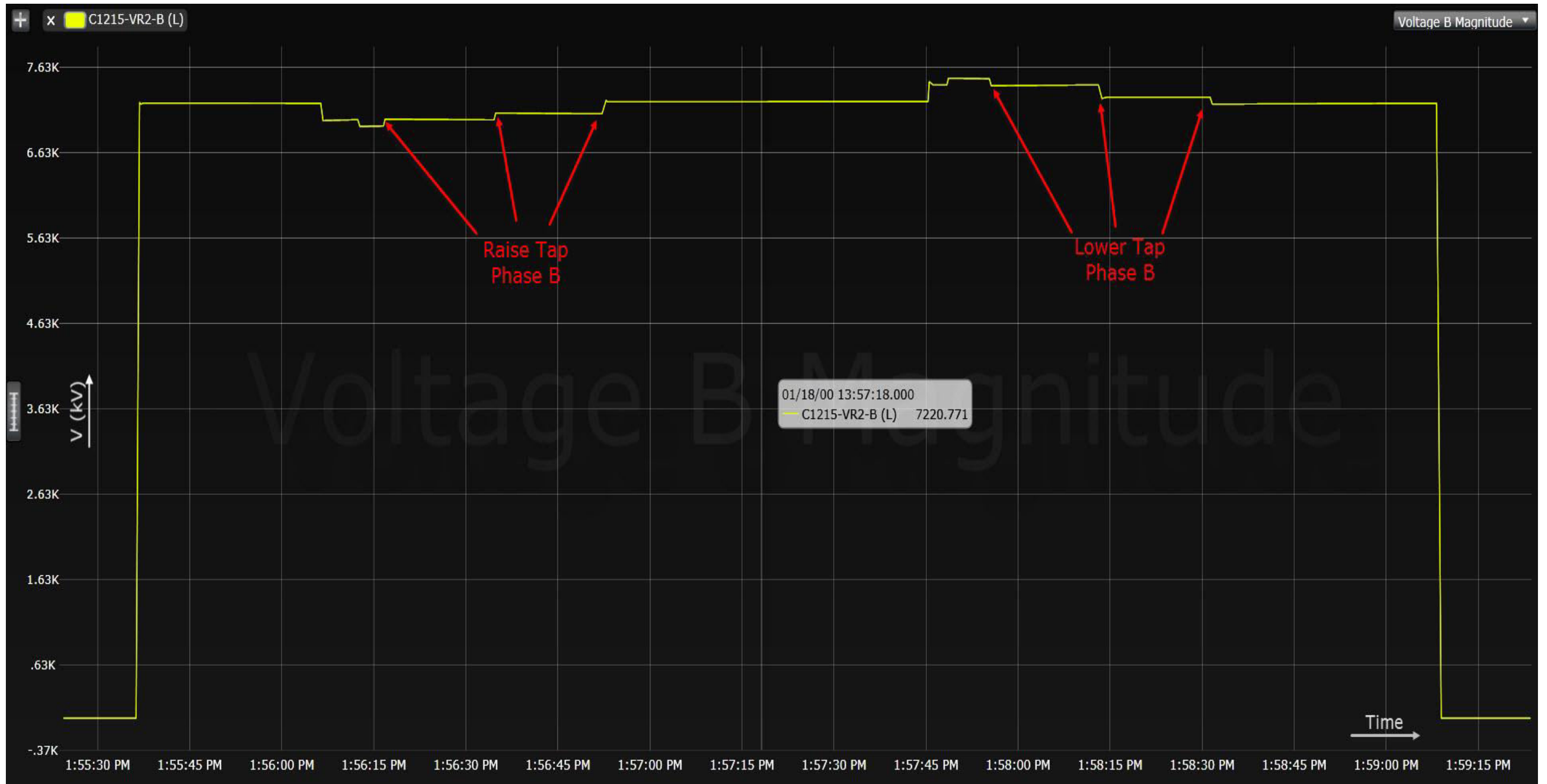
Figure 6.16: Test Scenario 3.7.2. Phase B Voltage Regulator Output Voltage Waveform
