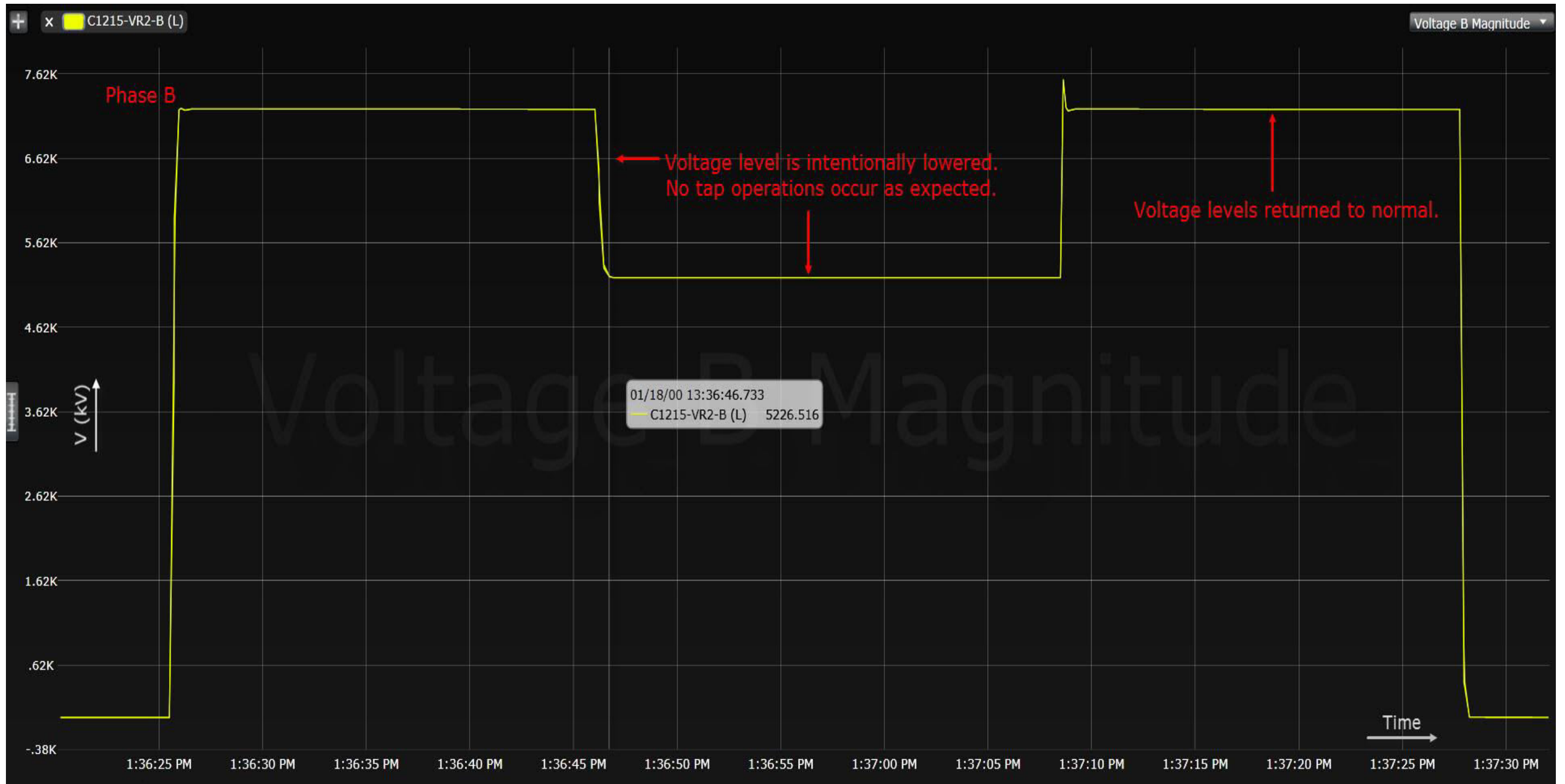
Figure 6.22: Test Scenario 3.7.3. Phase B Voltage Regulator Output Voltage Waveform
