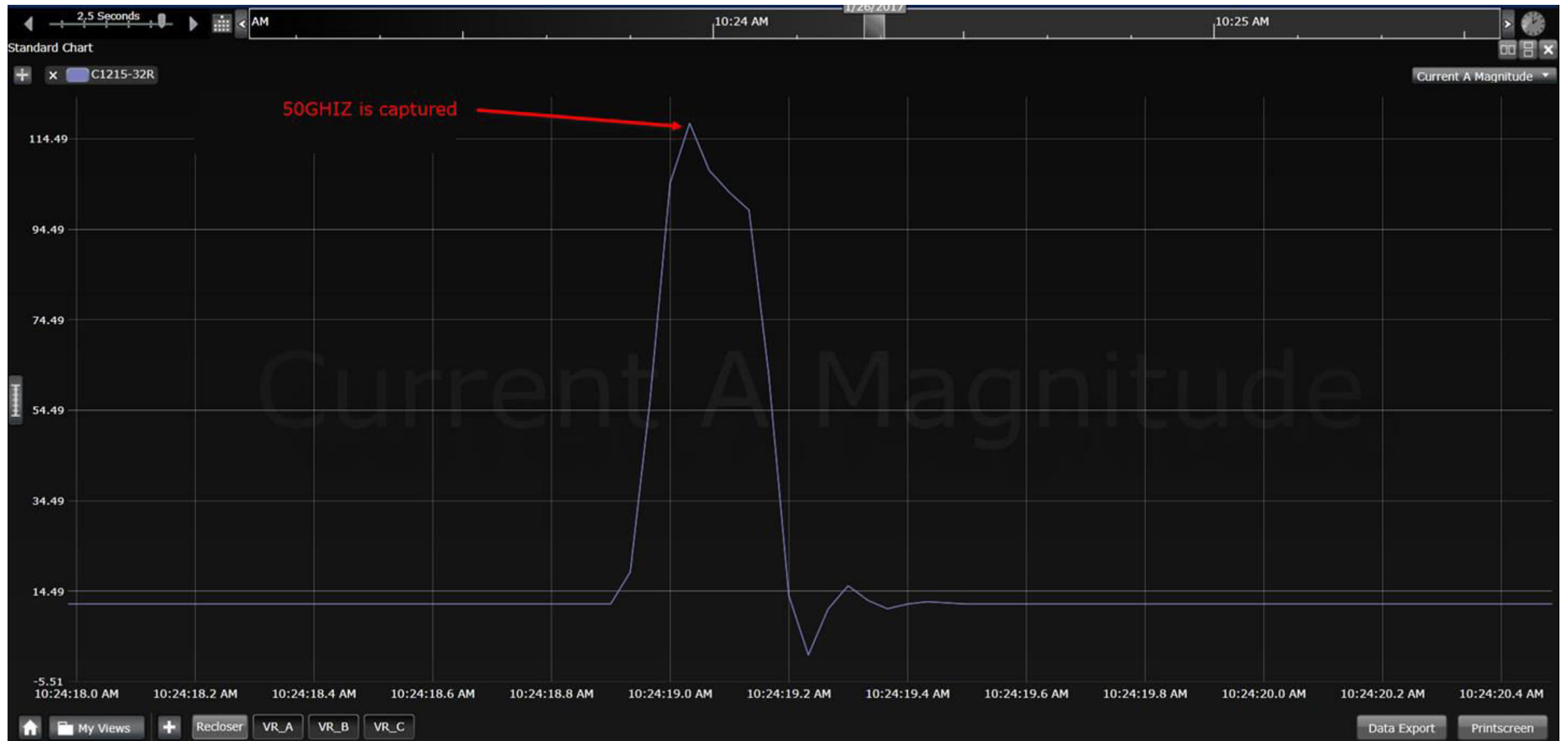
Figure 8.10: Scenario 1 – C1215-32R Current A Magnitude – Single Spike
