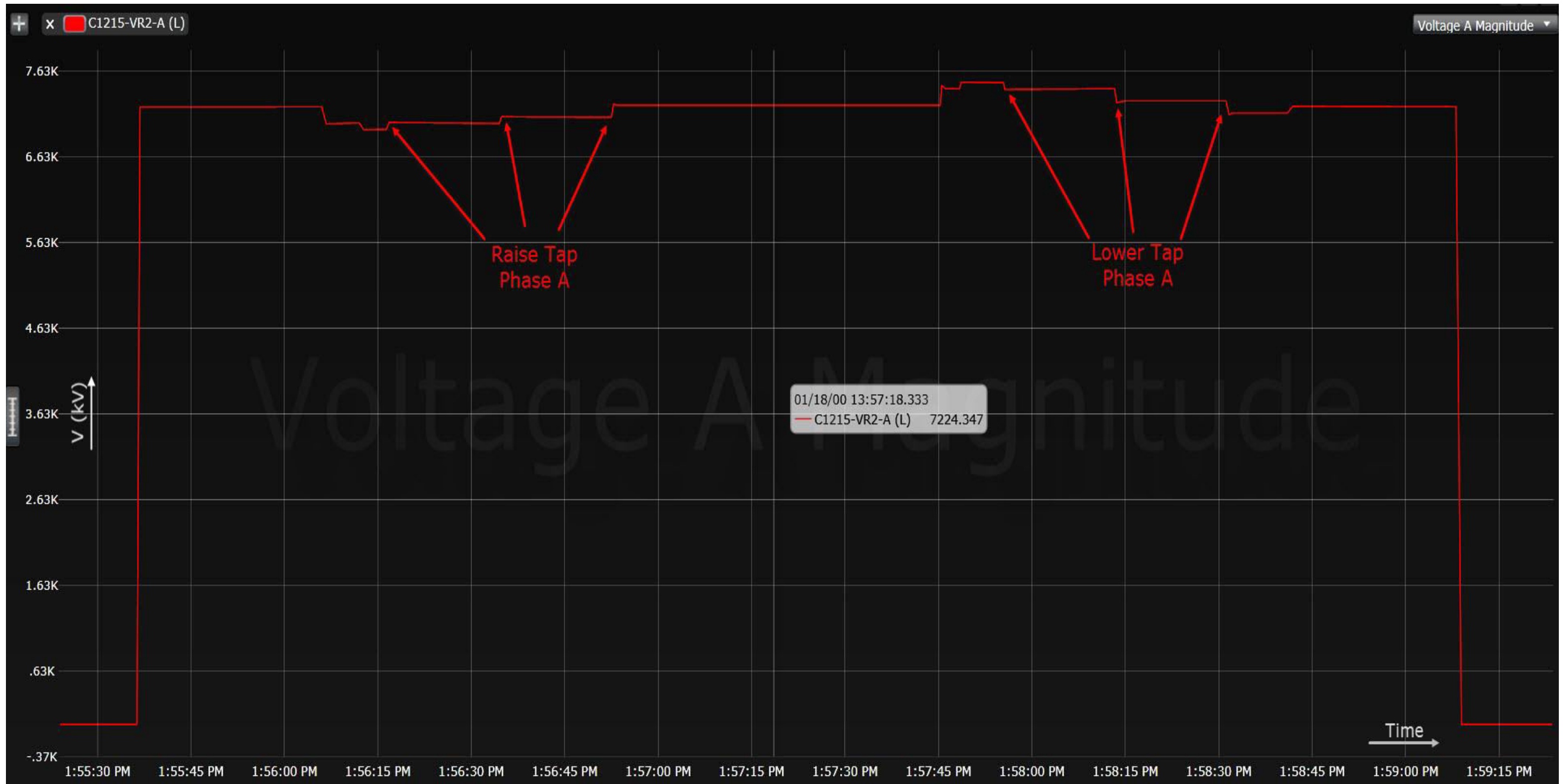
Figure 6.14: Test Scenario 3.7.2. Phase A Voltage Regulator Output Voltage Waveform
