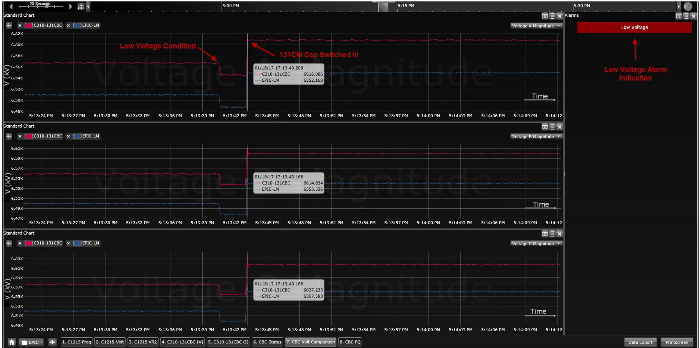
Figure 7.14: CBC Low-Voltage Condition
