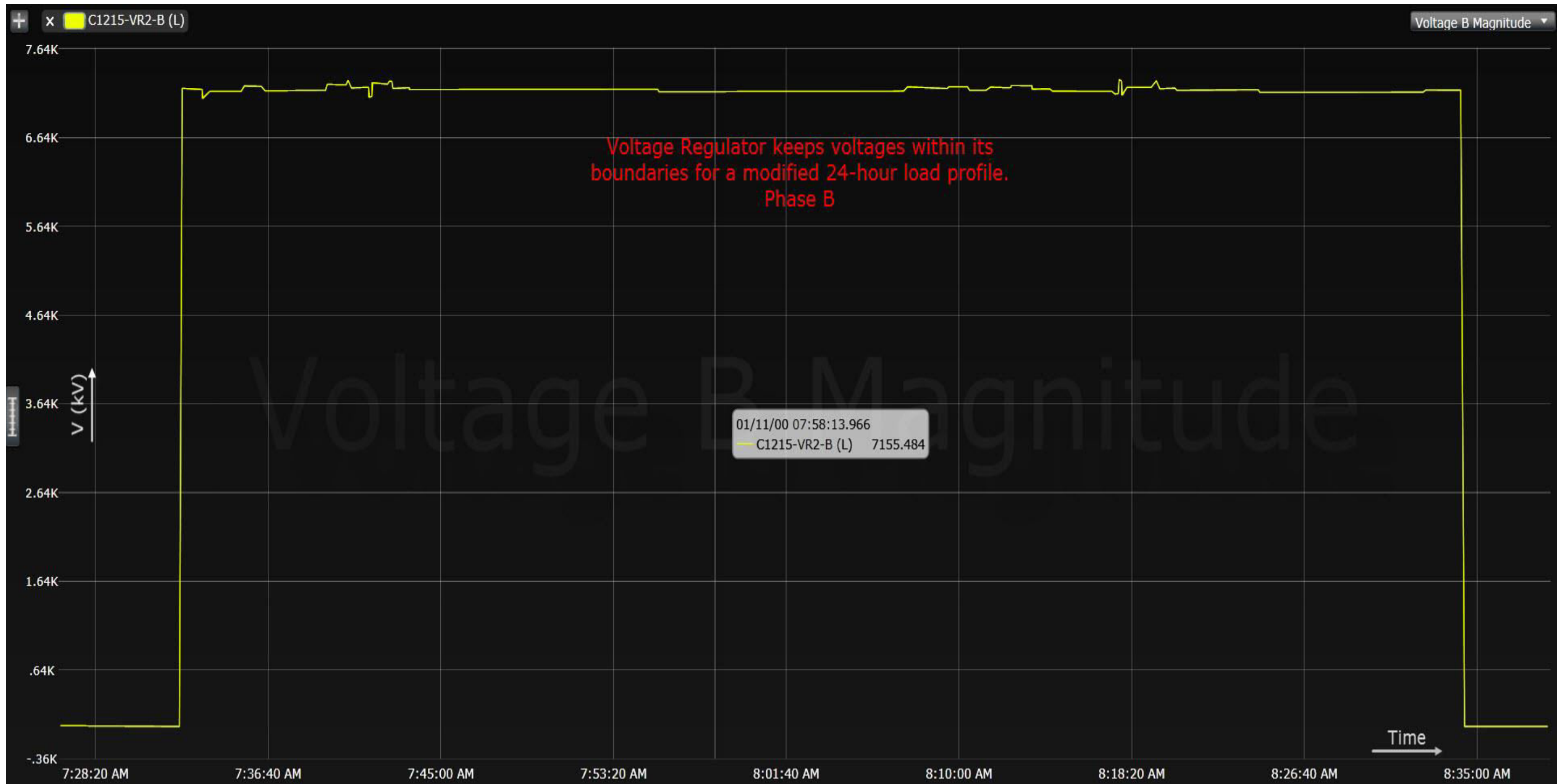
Figure 6.30: Test Scenario 3.7.4. Phase B Voltage Regulator Output Voltage Waveform – Modified Load Profile
