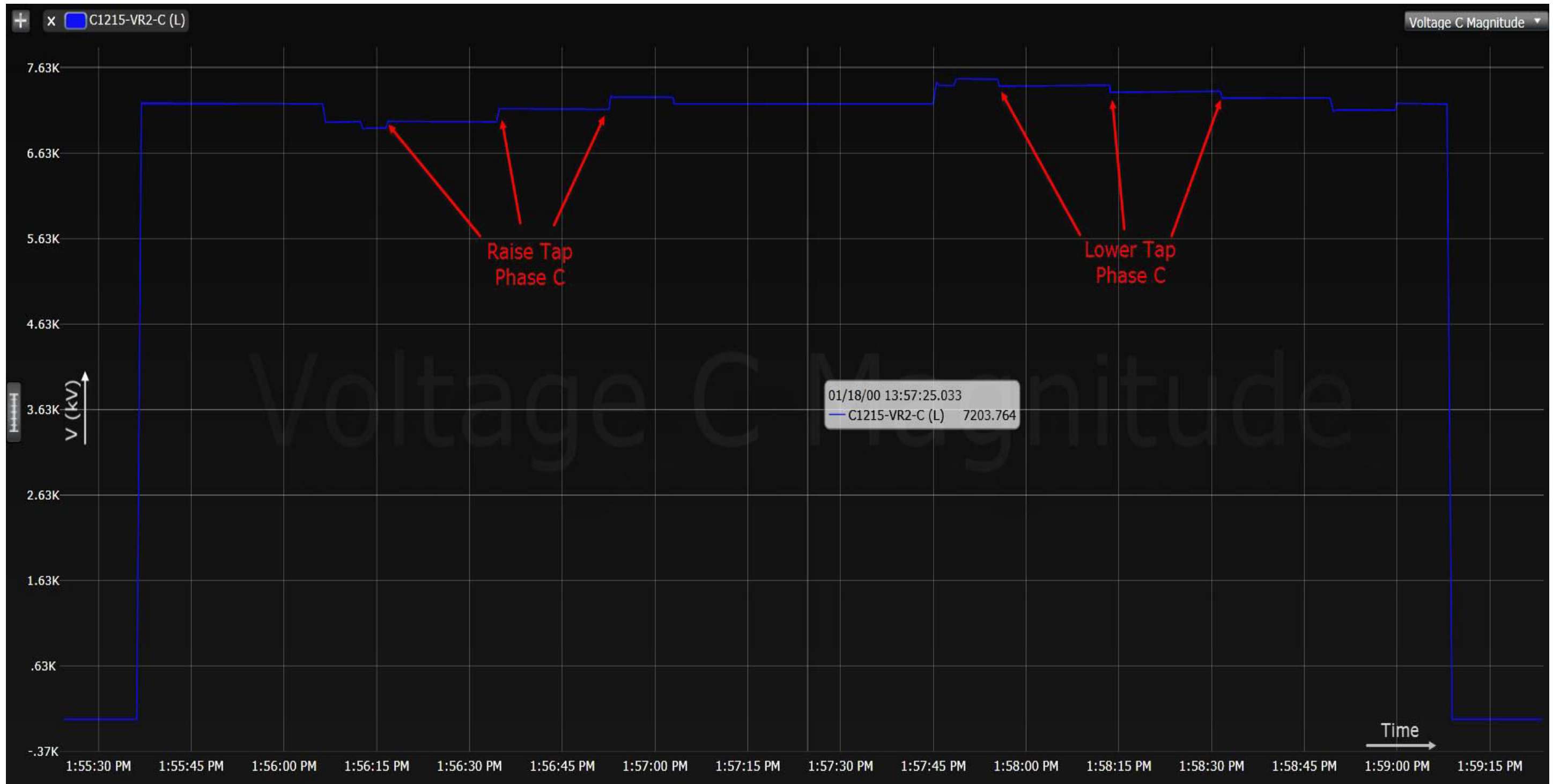
Figure 6.18: Test Scenario 3.7.2. Phase C Voltage Regulator Output Voltage Waveform
