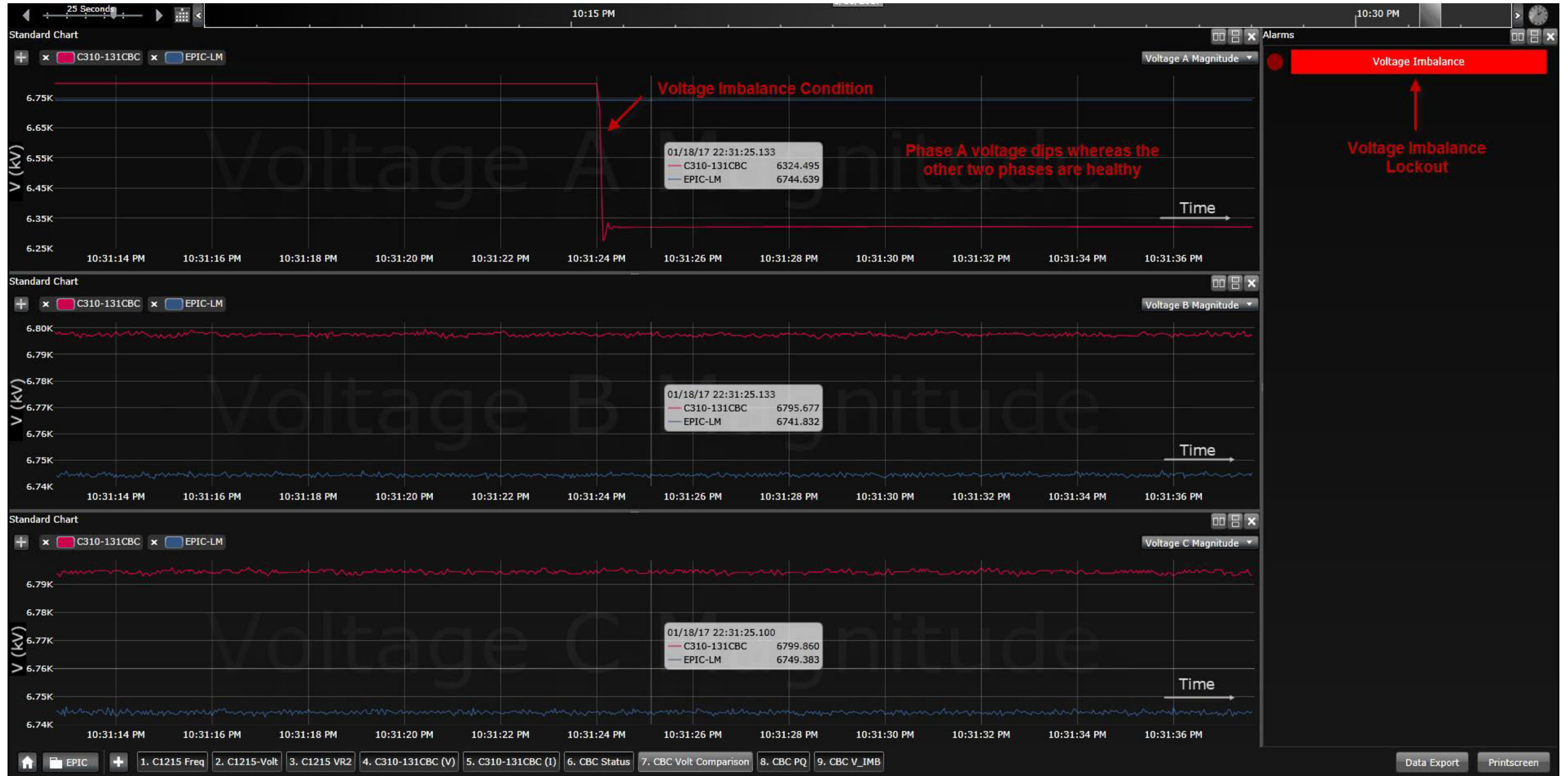
Figure 7.27: CBC Voltage Imbalance Condition
