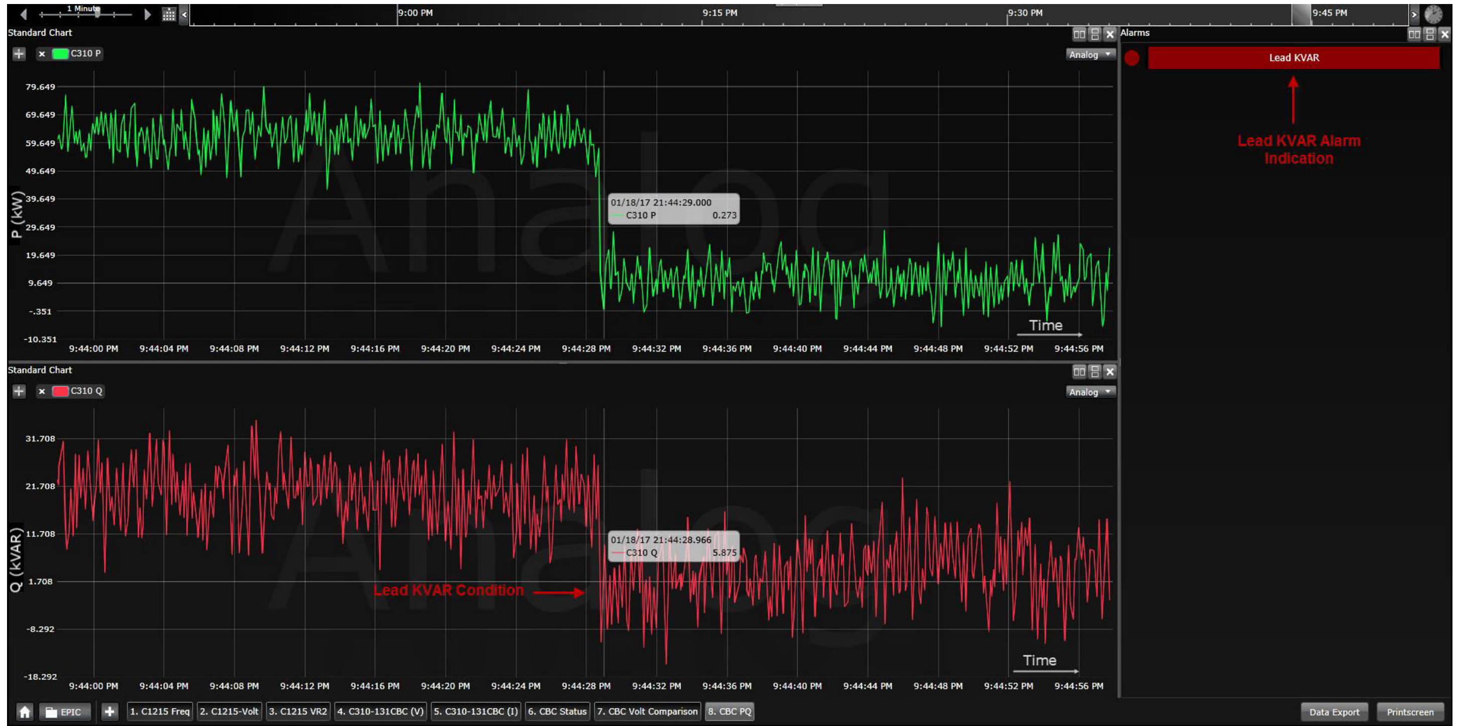
Figure 7.16: CBC Lead KVAR Condition – PQ Plot
