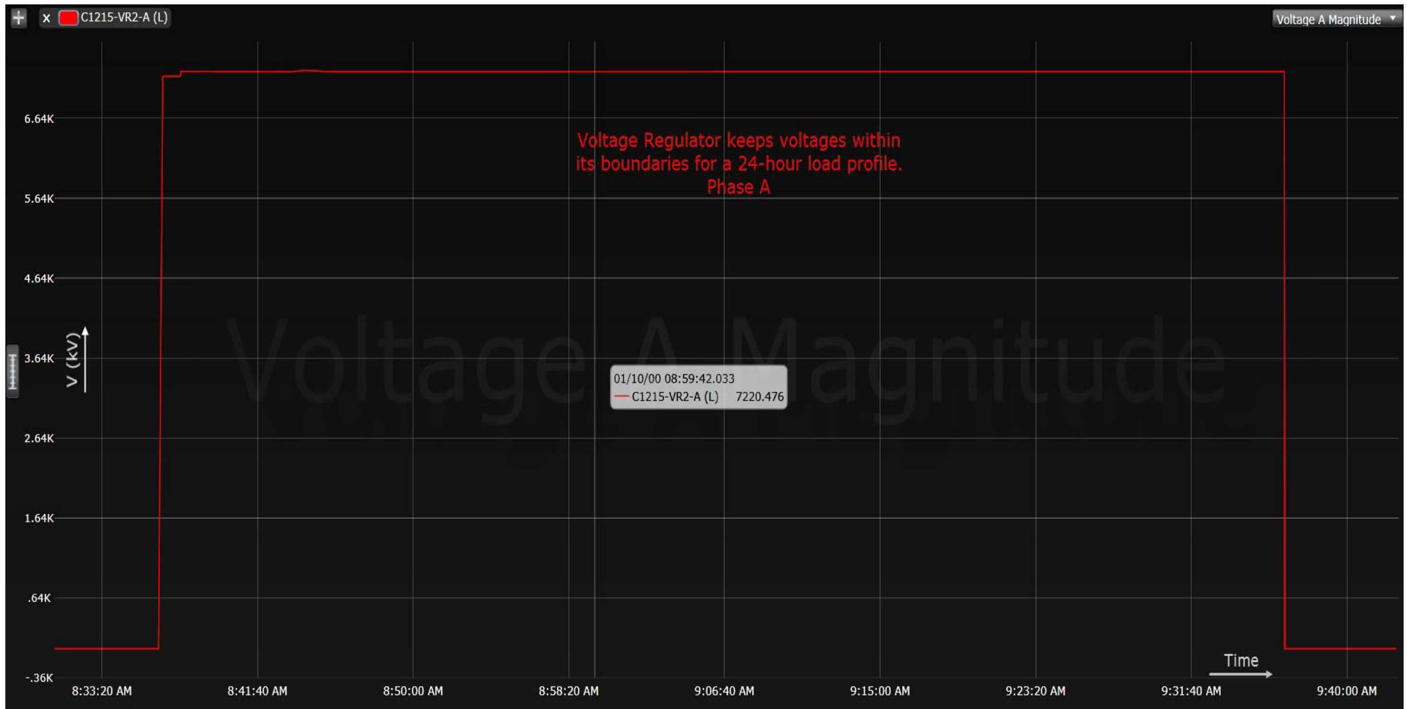
Figure 6.26: Test Scenario 3.7.4. Phase A Voltage Regulator Output Voltage Waveform – Normal Load Profile
