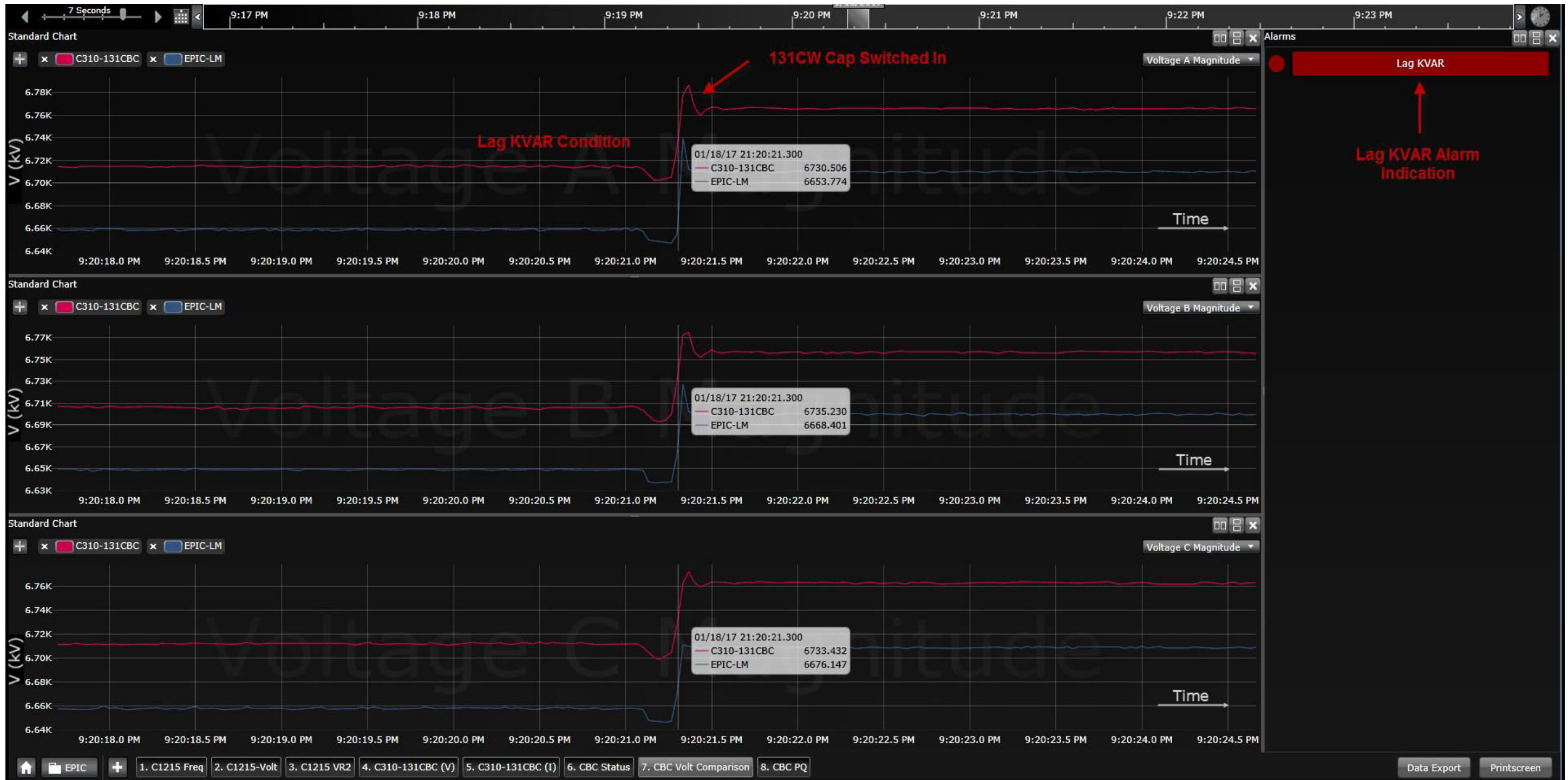
Figure 7.20: CBC Lag KVAR Condition – Voltage Plot
