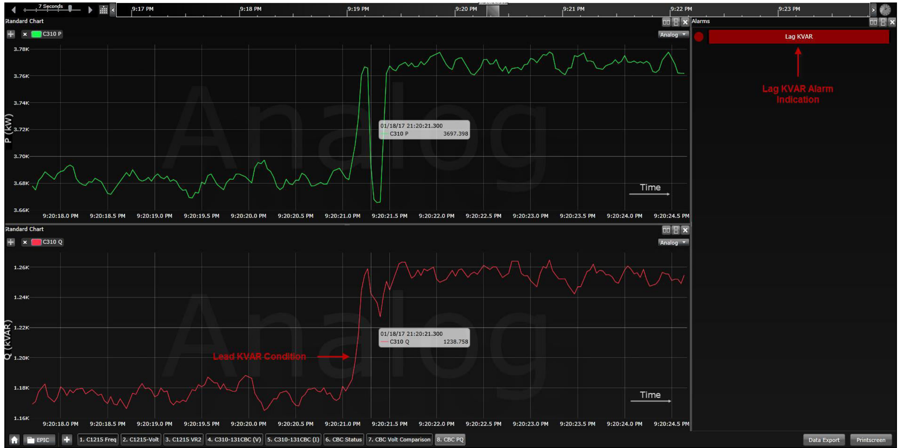
Figure 7.19: CBC Lag KVAR Condition – PQ Plot
