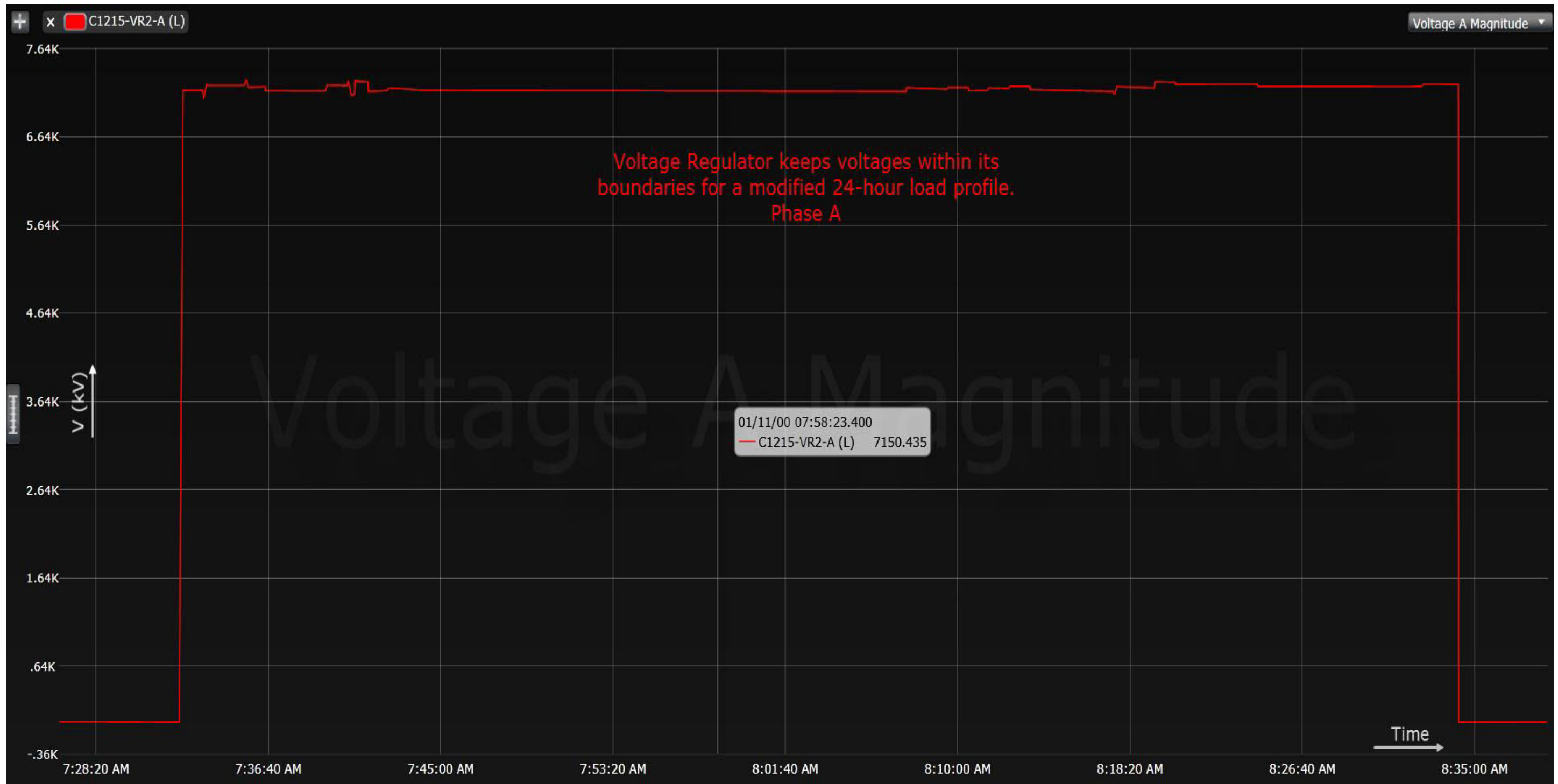
Figure 6.28: Test Scenario 3.7.4. Phase A Voltage Regulator Output Voltage Waveform – Modified Load Profile
