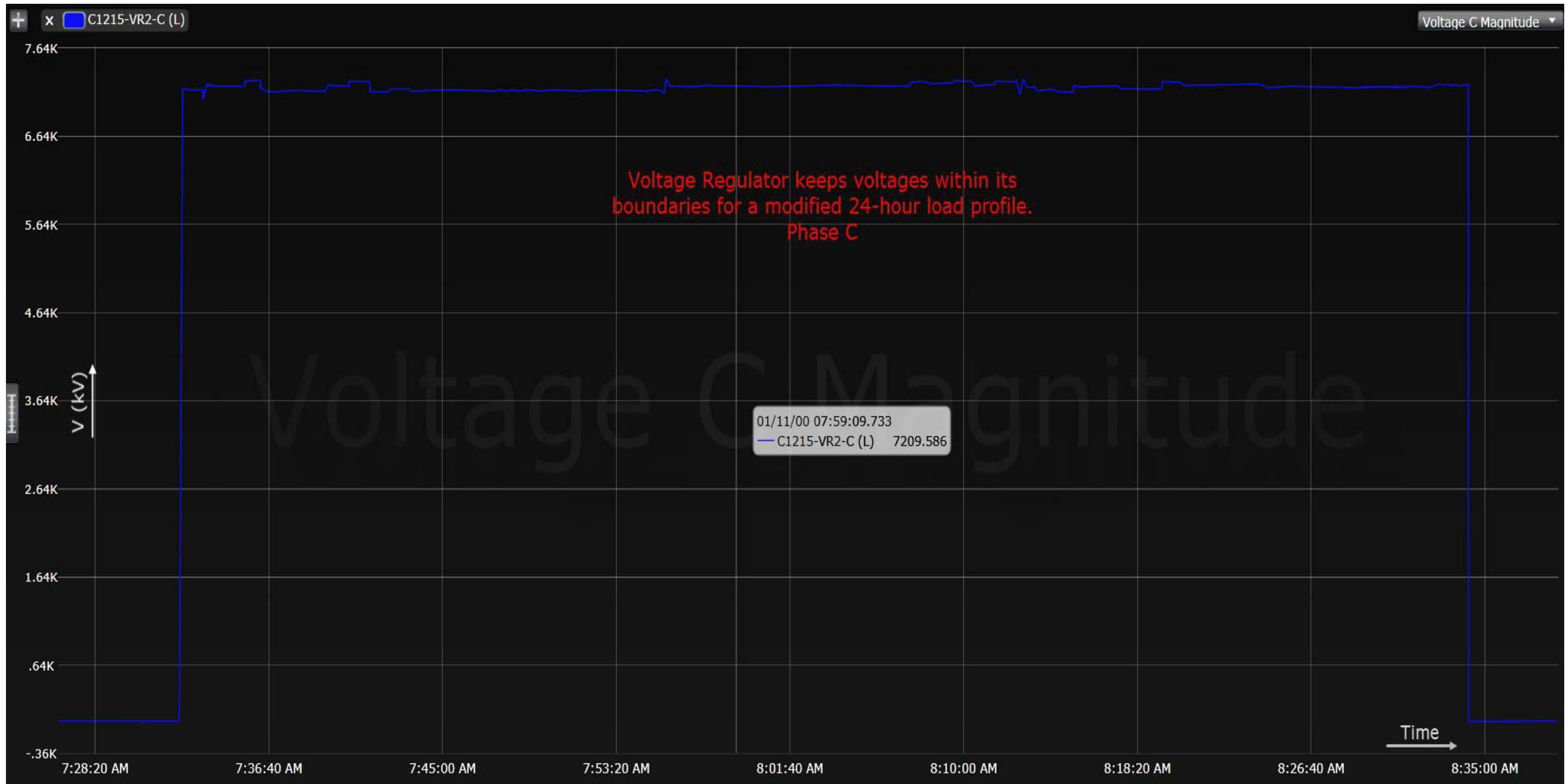
Figure 6.32: Test Scenario 3.7.4. Phase C Voltage Regulator Output Voltage Waveform – Modified Load Profile
