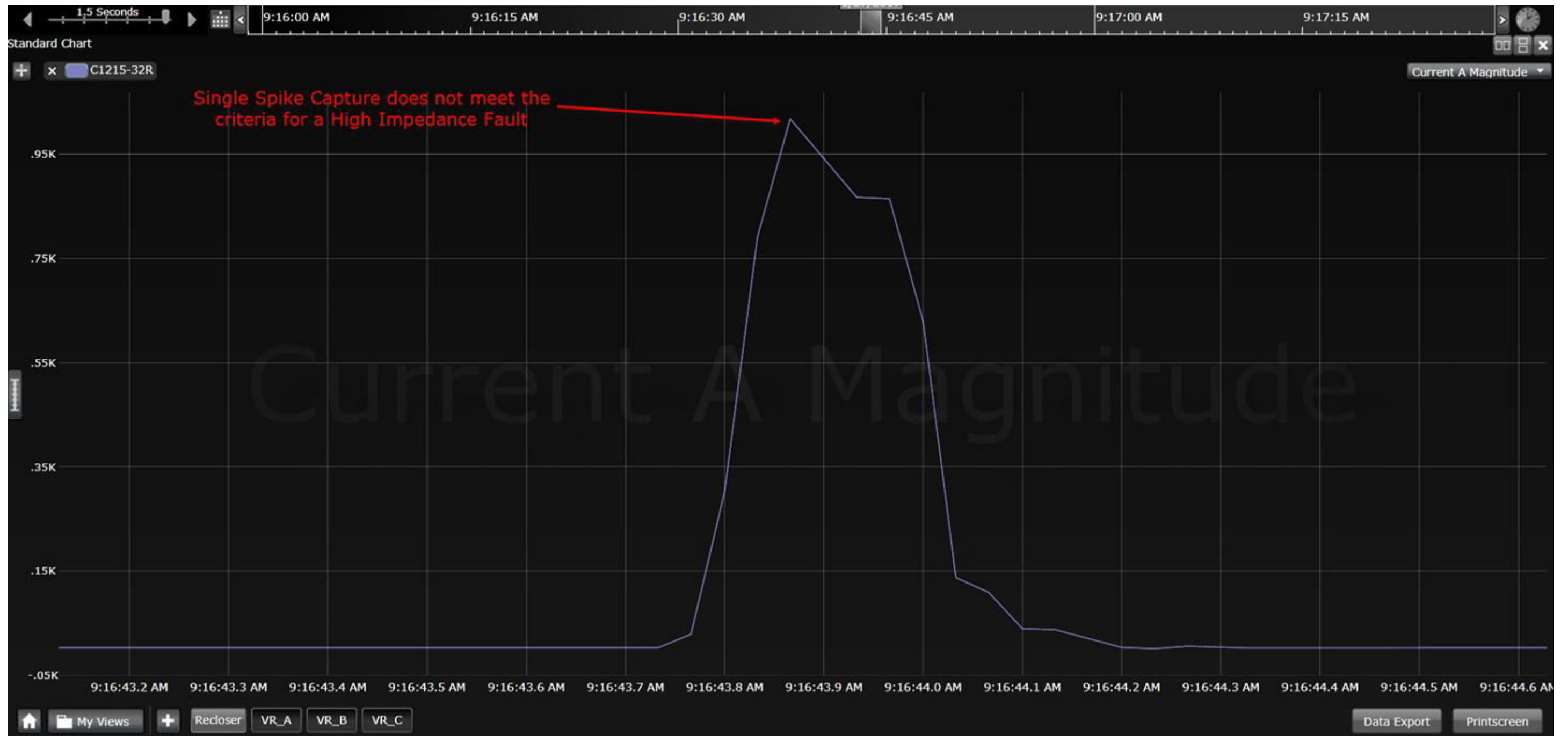
Figure 8.18: Scenario 4 – Central Single Spike Does Not Meet HIF Criteria
