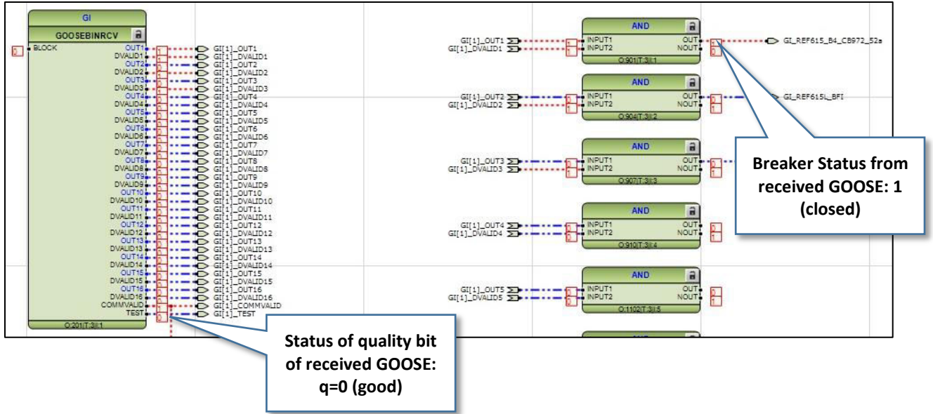
Figure D-16. Online status of received GOOSE (q=good) in REC670 (mode=on)
