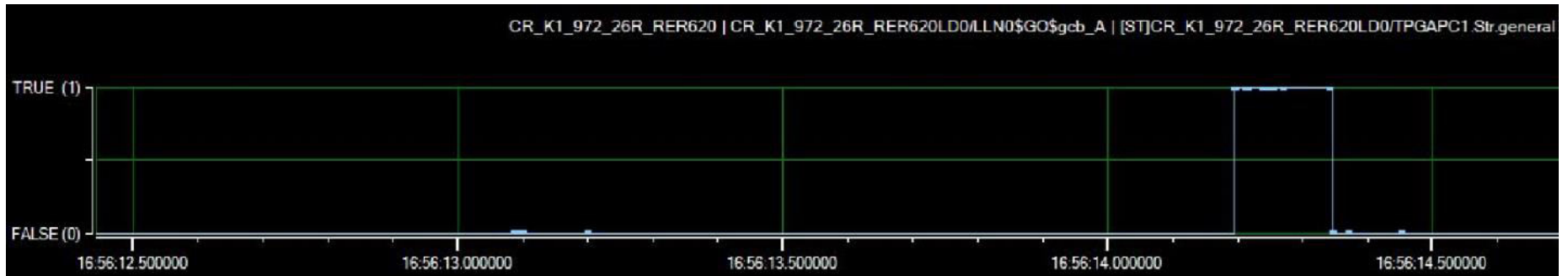
Figure 2-16. A binary GOOSE message sent by RER620 to trip CCR2-32R for a downstream feeder fault
