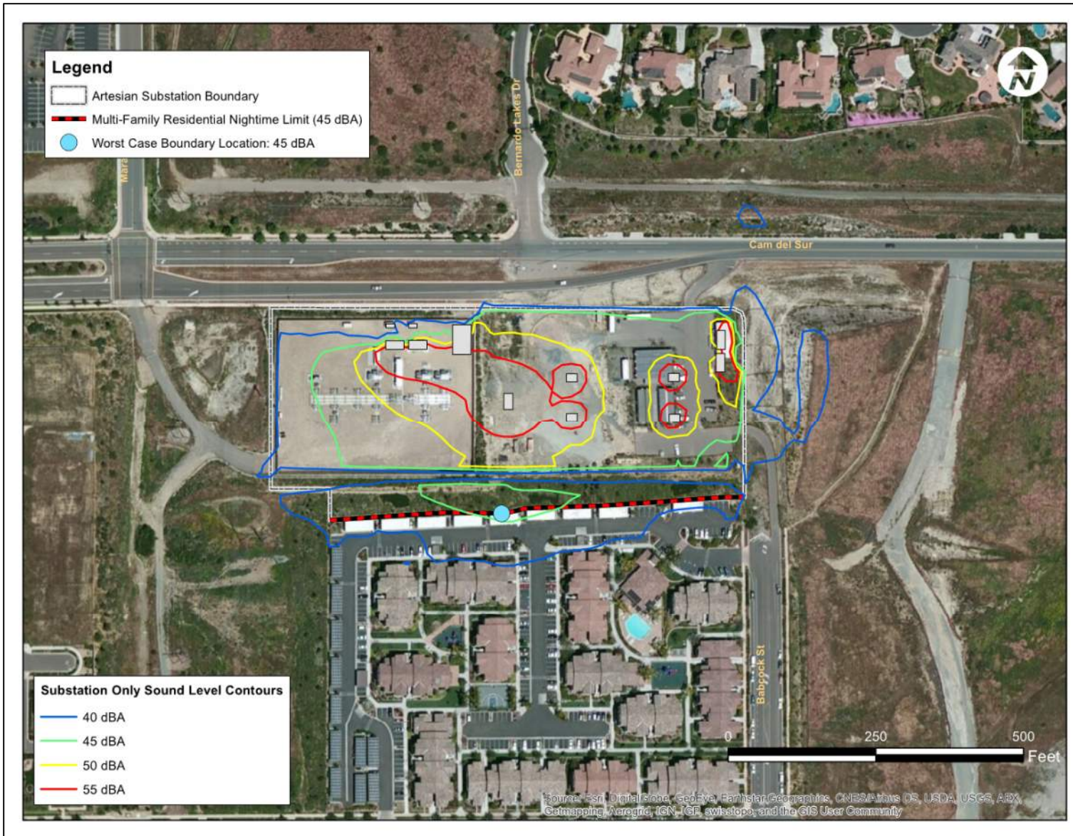
Figure 3-2 Substation (only) sound pressure levels.
