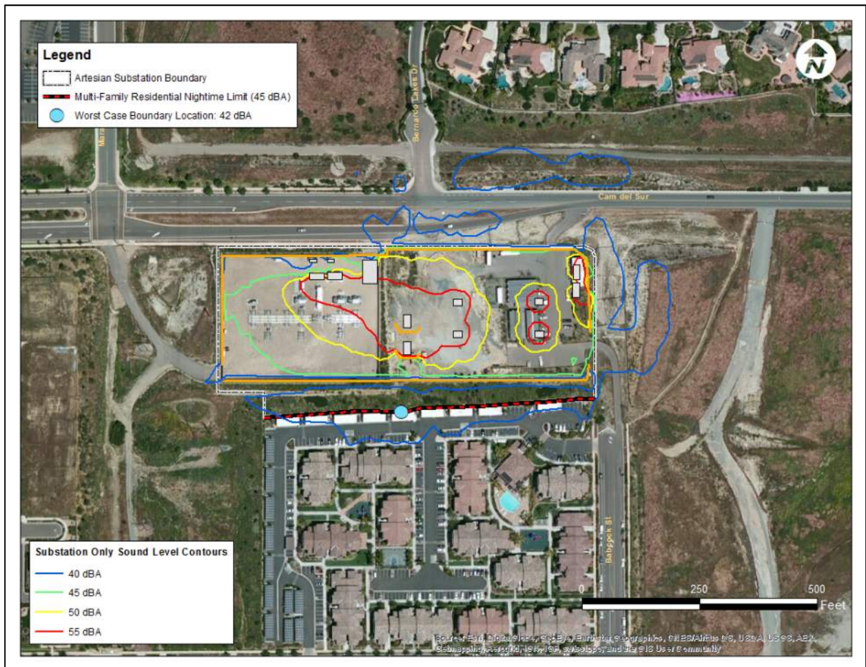
Figure B-1 Mitigation Alternative - Noise barrier wall arrangement
