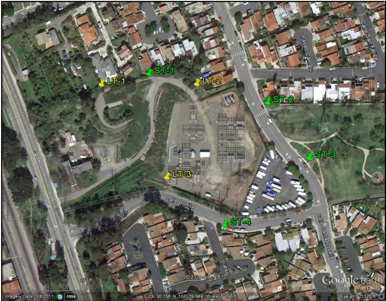
Figure 3 - Ambient Noise Measurement Locations at the Capistrano Substation [Long-term locations shown in yellow, short-term locations shown in green]
