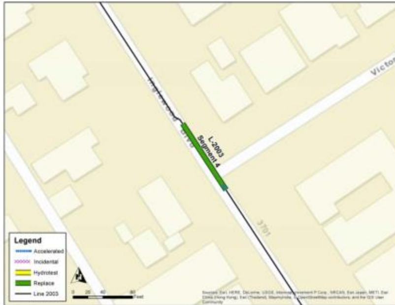
Figure 7: Overview Map of L-2003 Section 4 Replacement Project
