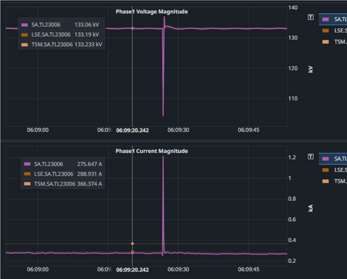
2/15/24 230kV Line Fault Event: Current and Voltage from PMU
