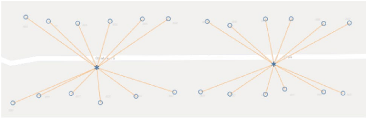
Figure 1. Typical meter-to-transformer connectivity on a suburban street
