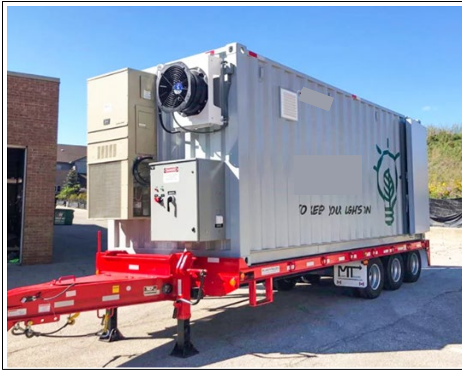
Figure 3-2. MBESS Container used in the project
